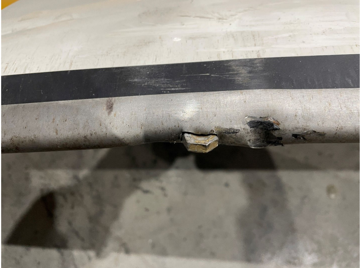
Figure 2: Bolt Head from tail rotor embedded in main rotor blade
