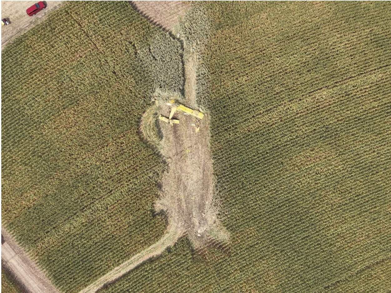
Figure 4 - Overhead photo of the initial ground impact and main wreckage. (Photo courtesy of Morgan County Sheriff's Office)
