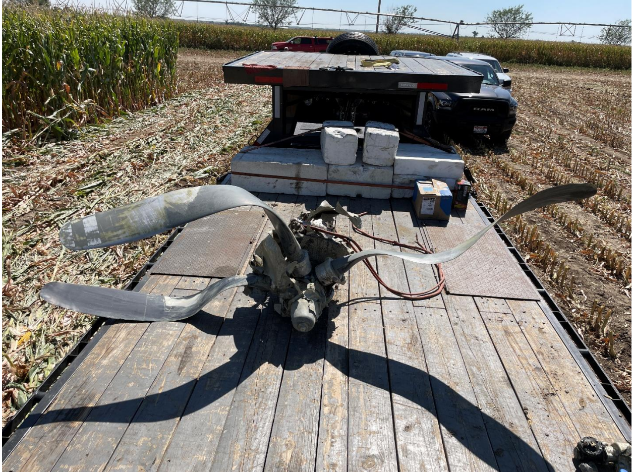
Figure 13 - Propeller hub assembly with 3 blades attached after recovery.
