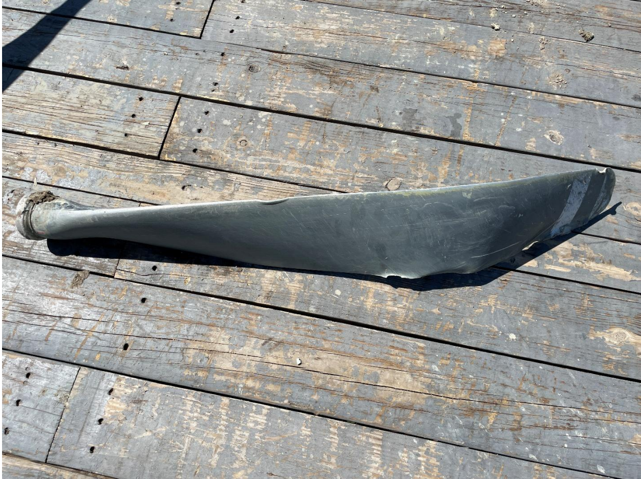
Figure 14 - Propeller blade found separated from hub assembly.
