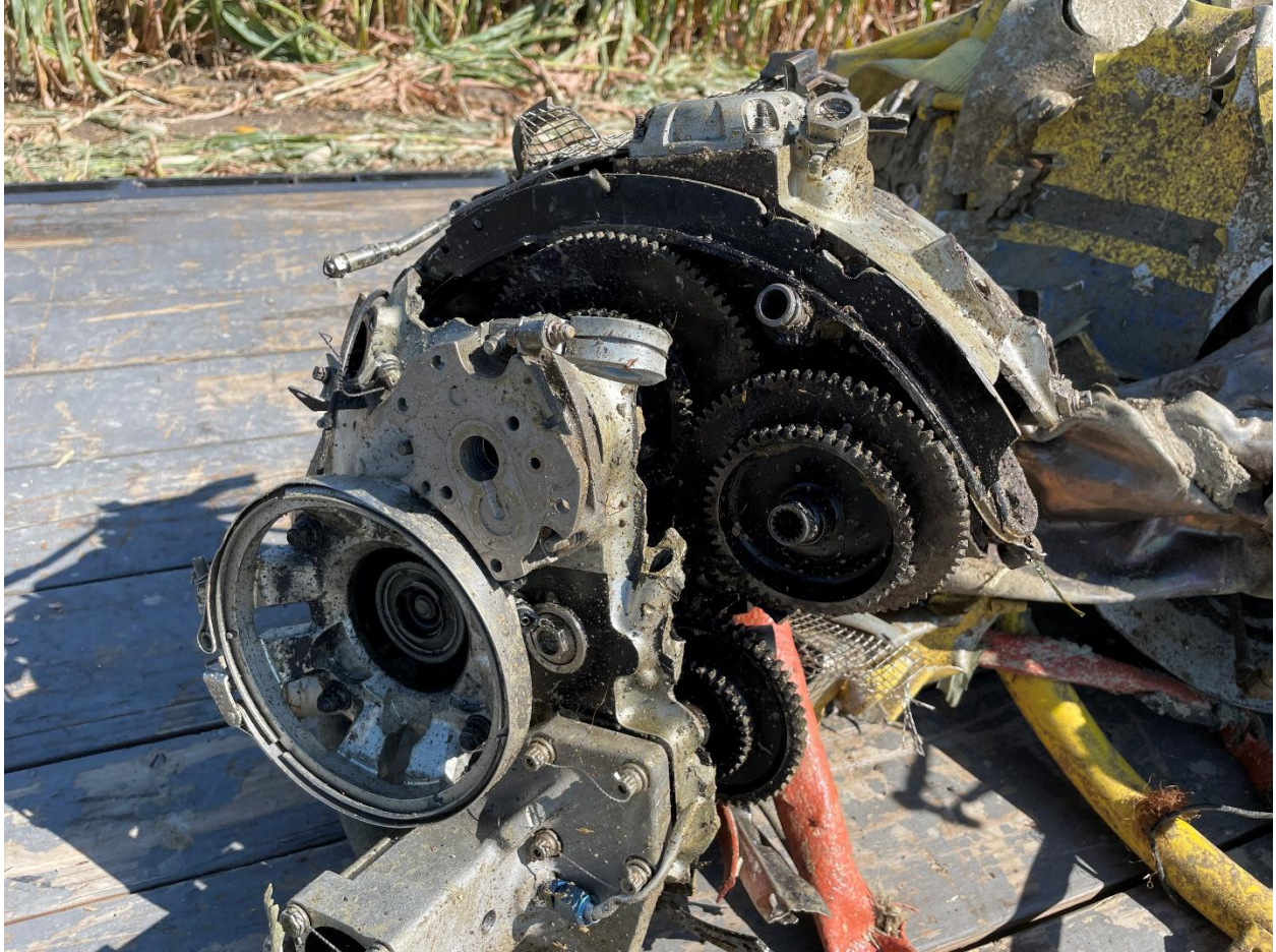
Figure 9 - Engine accessory gearbox.
