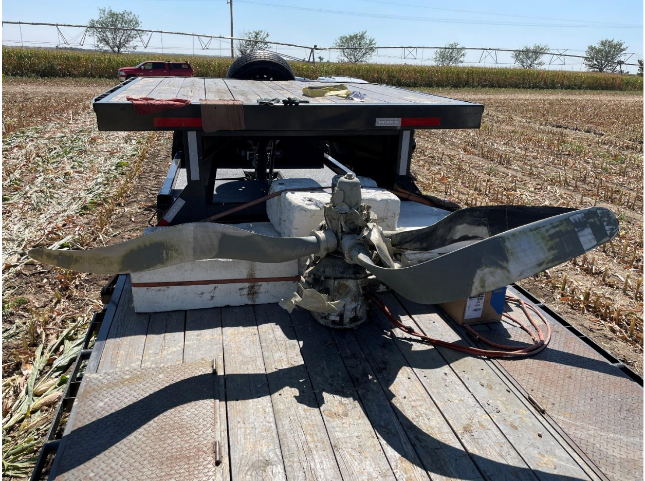
Figure 12 - Propeller hub assembly with 3 blades after recovery.
