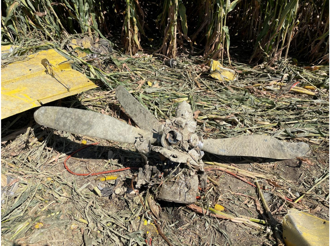
Figure 11 - Propeller hub assembly with 3 blades at the accident site.
