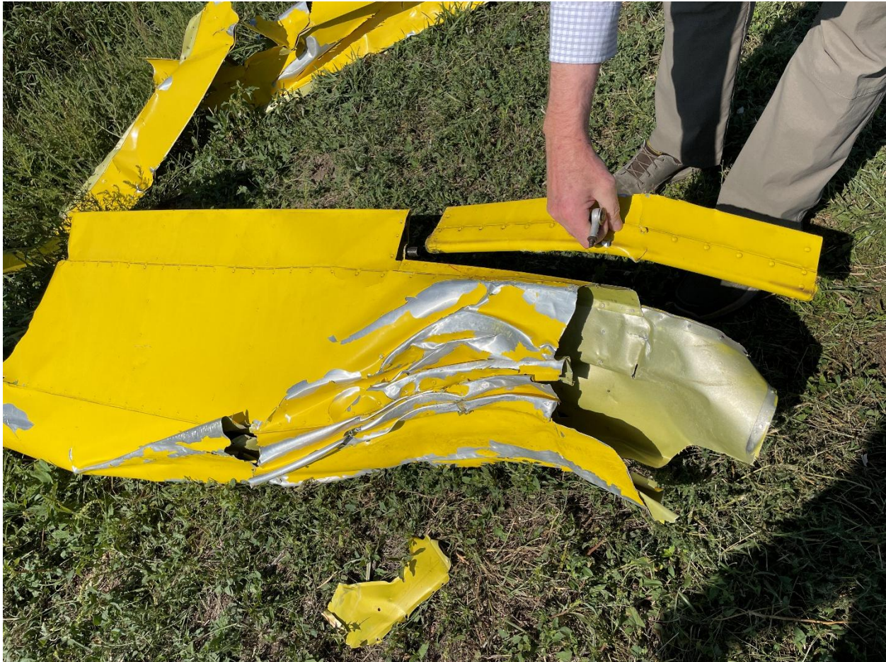
Figure 7 - Outboard 3 ft of right aileron and the aileron trim surface.
