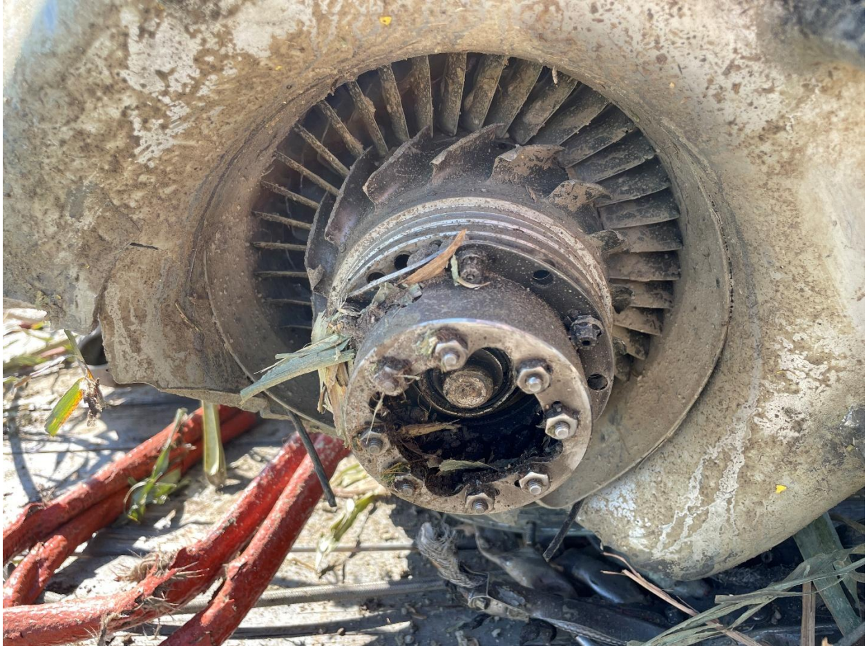
Figure 10 - Engine first stage compressor section.
