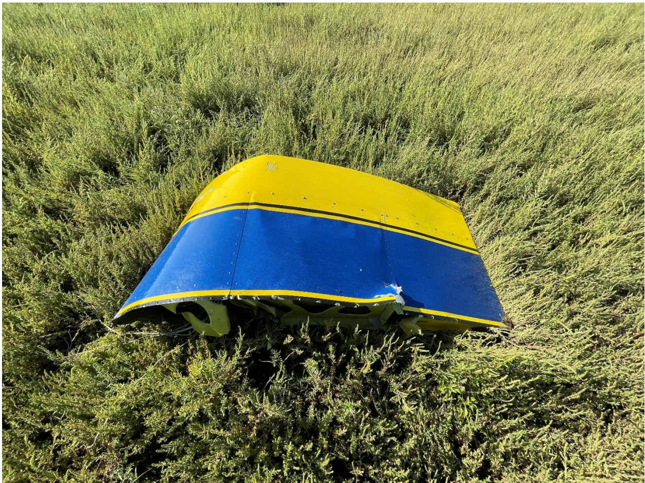
Figure 6 - Right wingtip as found along the wreckage debris path.
