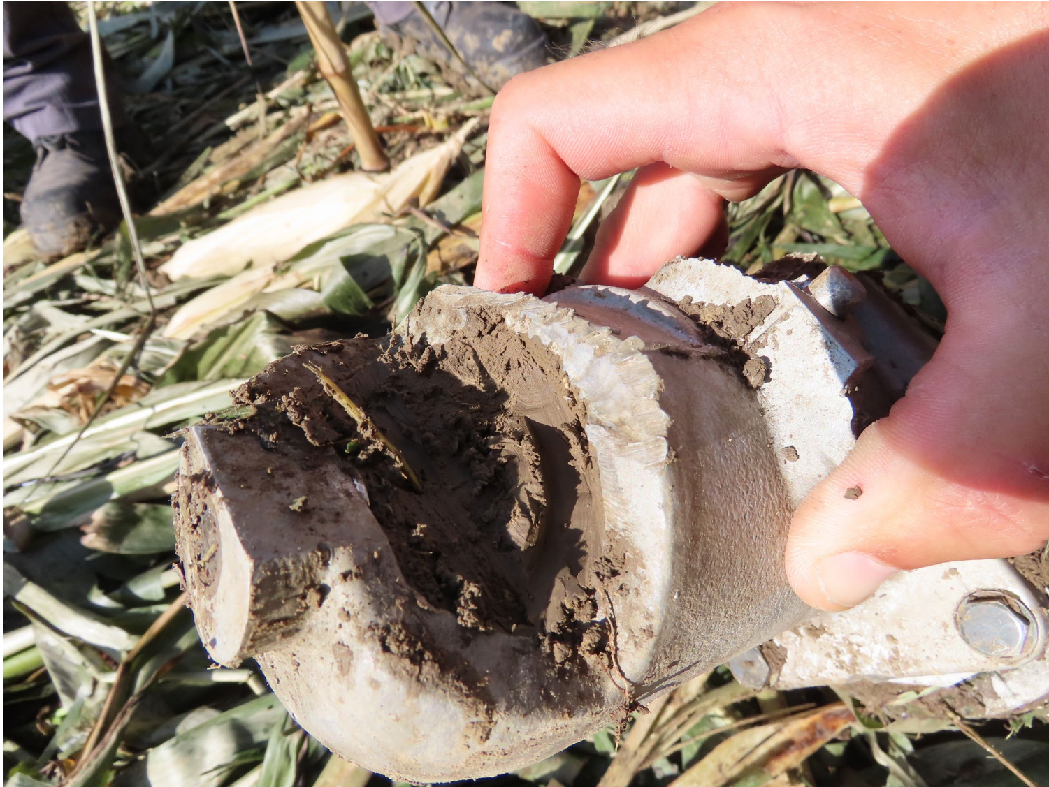
Photograph 5 - Starter motor impact signature
