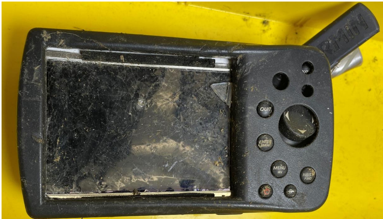
Figure 1. Photo of Garmin GPSMAP 396 showing impact damage.
