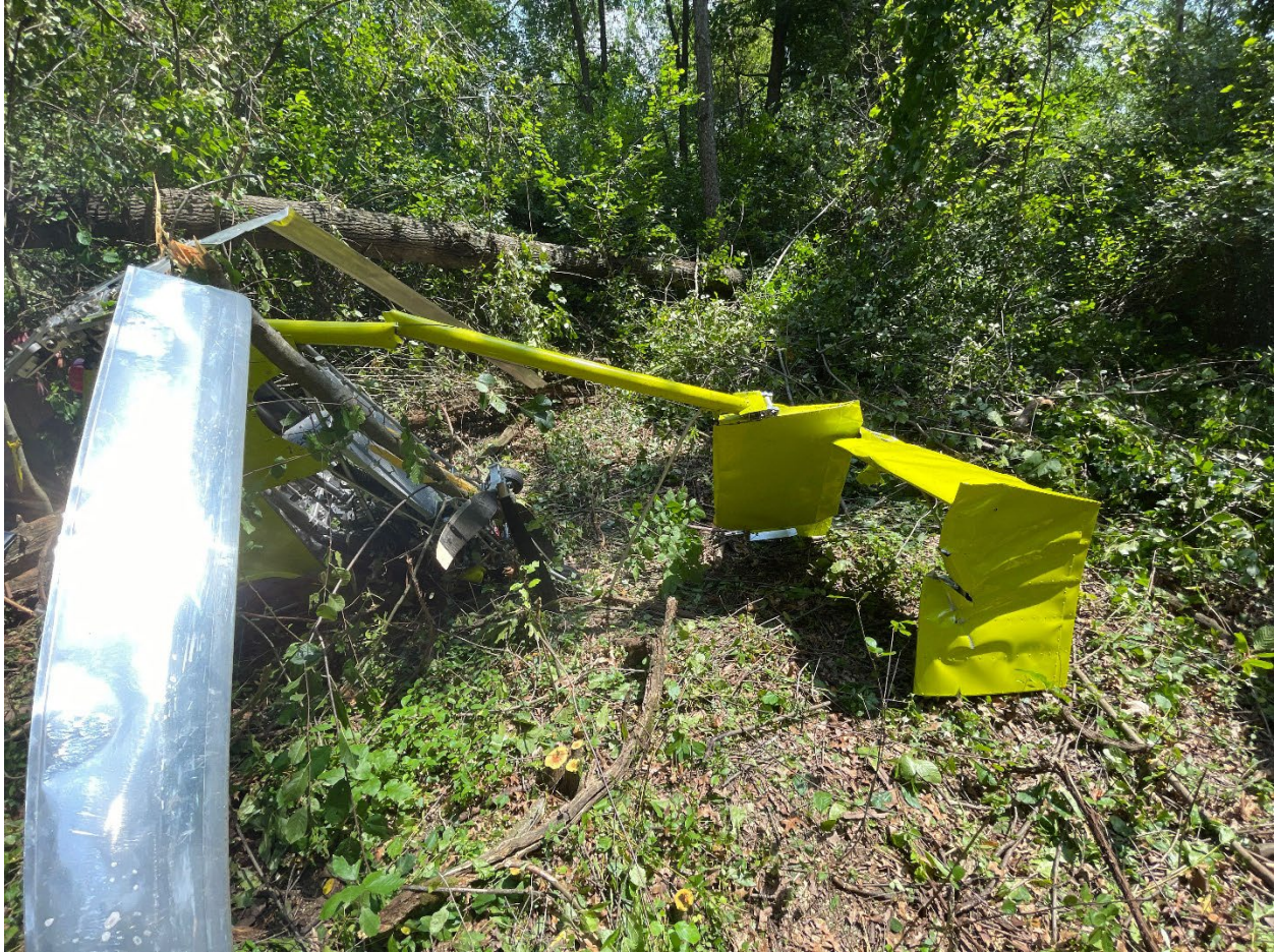
Figure 4. Tail surfaces and tail boom placed in pre-impact location.
