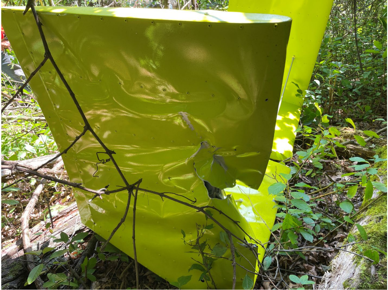
Figure 3. The gyroplane's tail surfaces with rotor impact mark.
