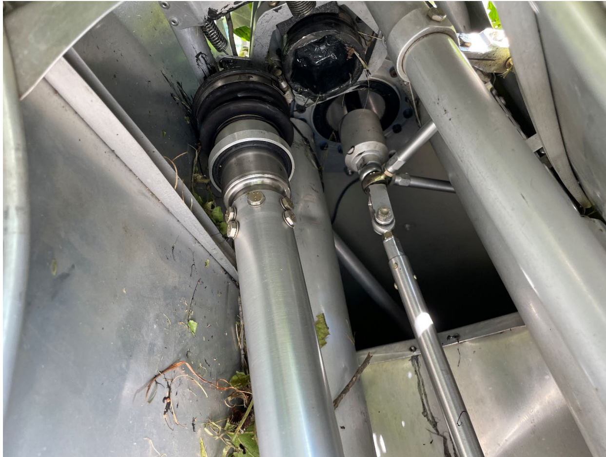
Photograph 4 - Separated rotor drive coupling (NTSB Photo)
