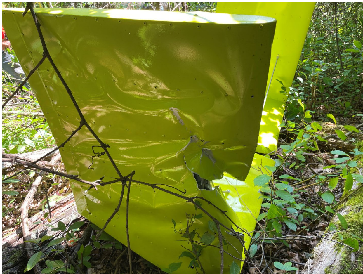
Photograph 2 - Tail surfaces showing rotor impact mark (NTSB Photo)
