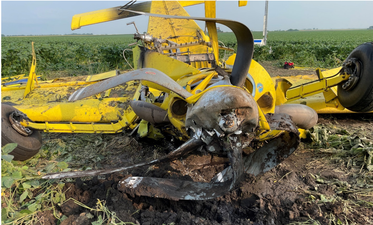
Figure 2. Damaged propeller blades after removal from the ground.
