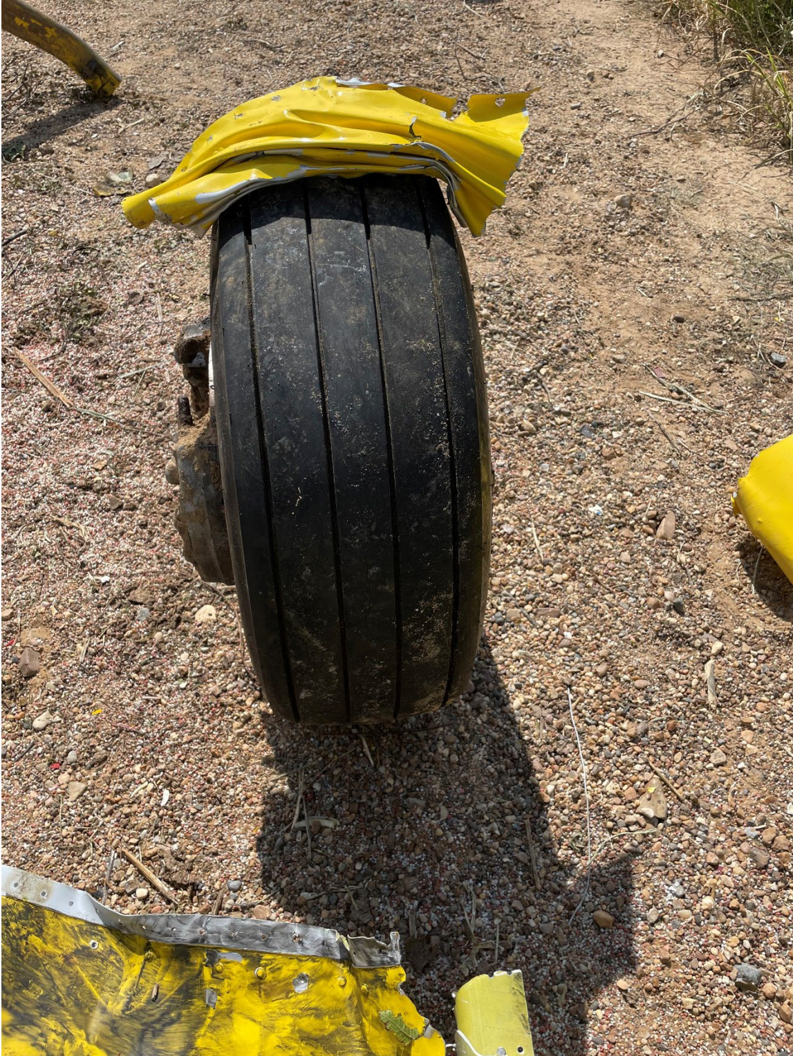
Figure 12. N6177J separated left wing structure with exemplar Air Tractor main landing gear wheel/tire.
