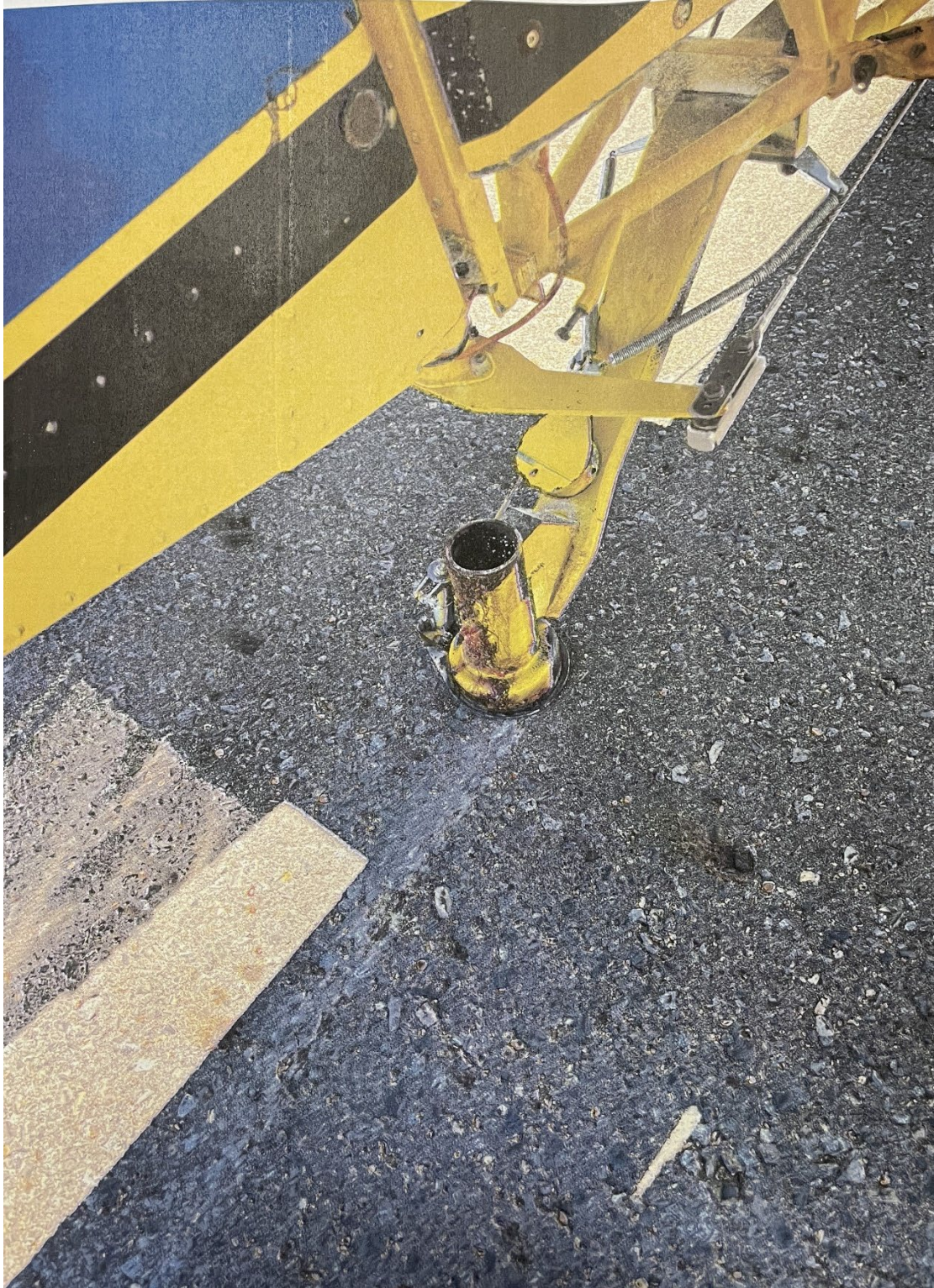
Figure 5. Missing tail wheel assembly following landing after the collision (Source: Arkla Flyers, Inc.)
