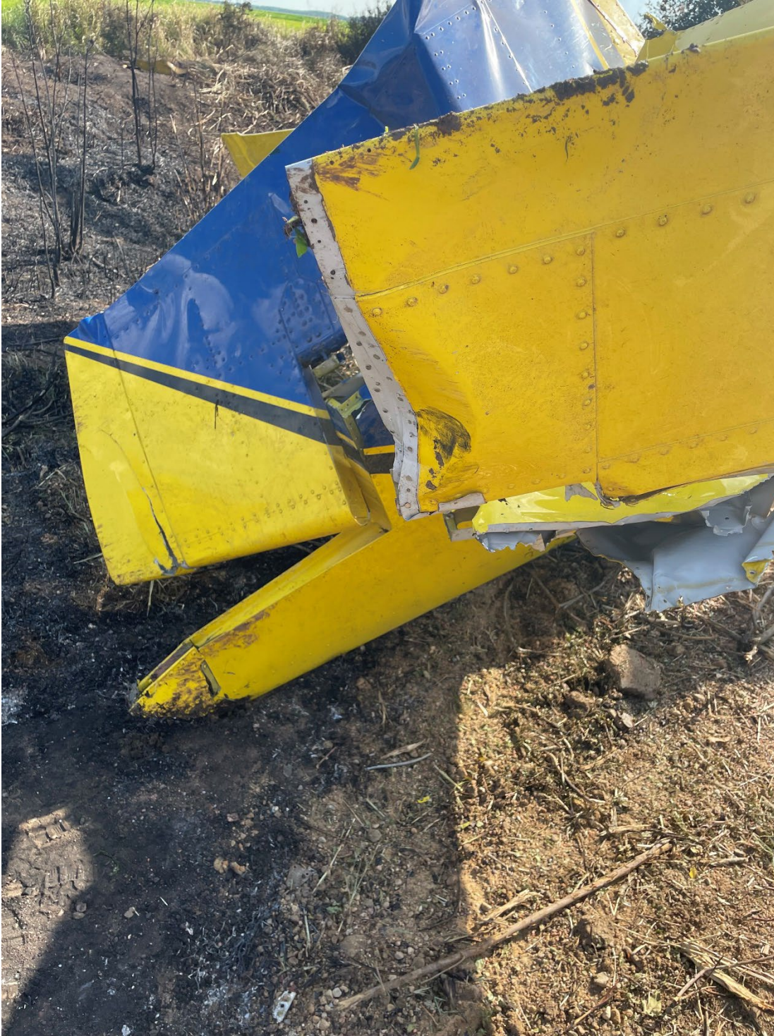
Figure 13. N6177J left horizontal stabilizer with black rubber transfer mark.
