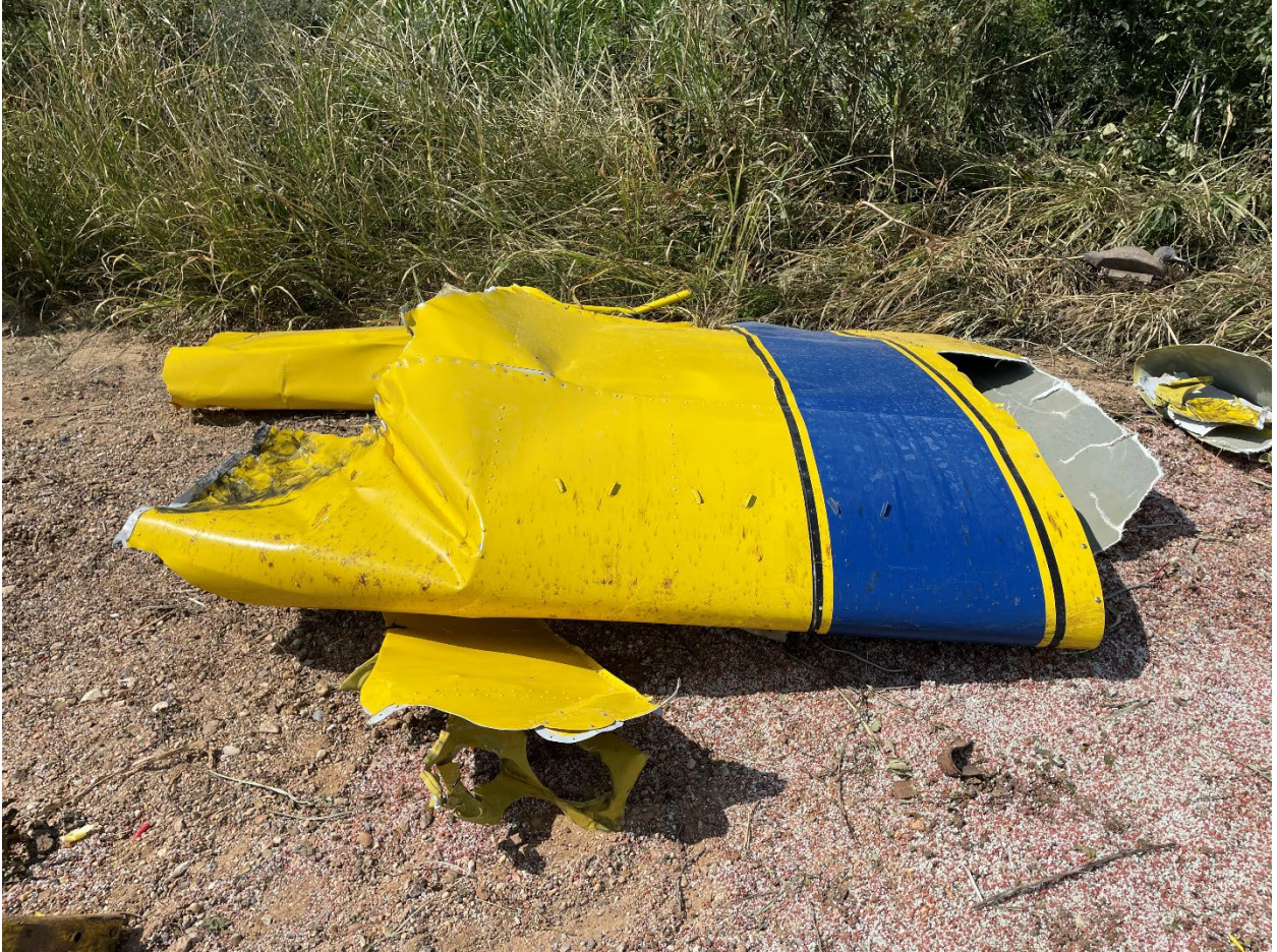
Figure 11. N6177J separated outboard left wing structure.
