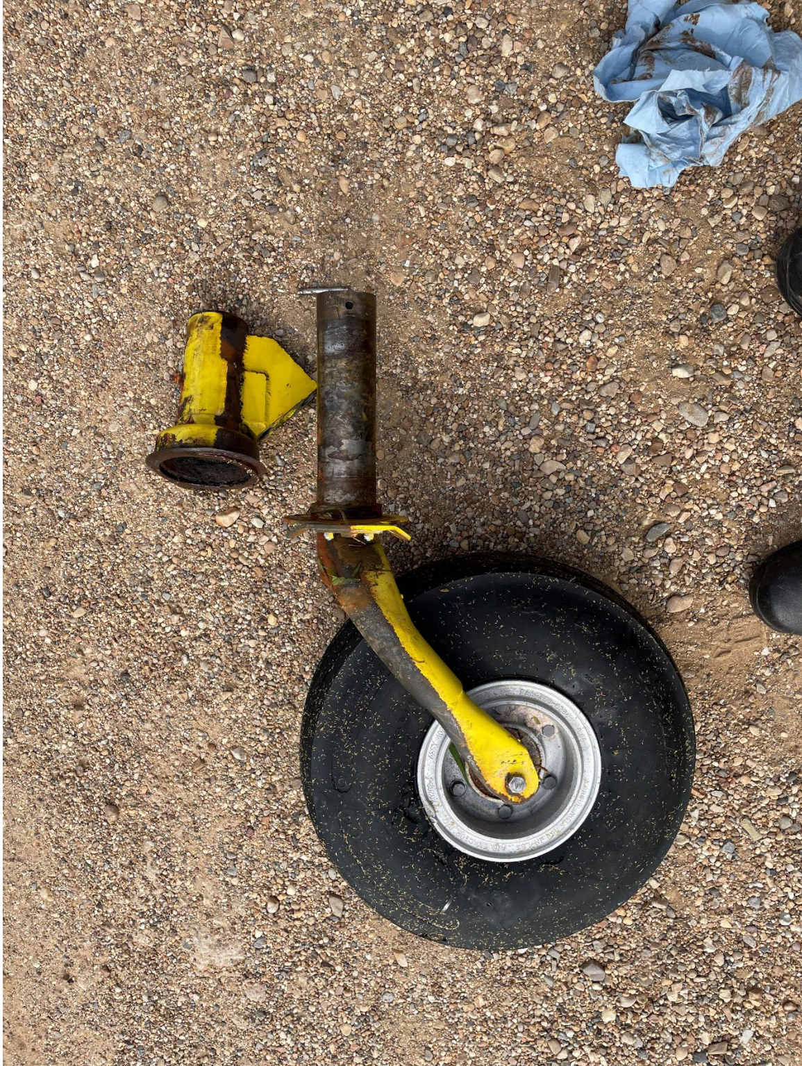
Figure 6. Accident tail wheel assembly after recovery from the rice field.
