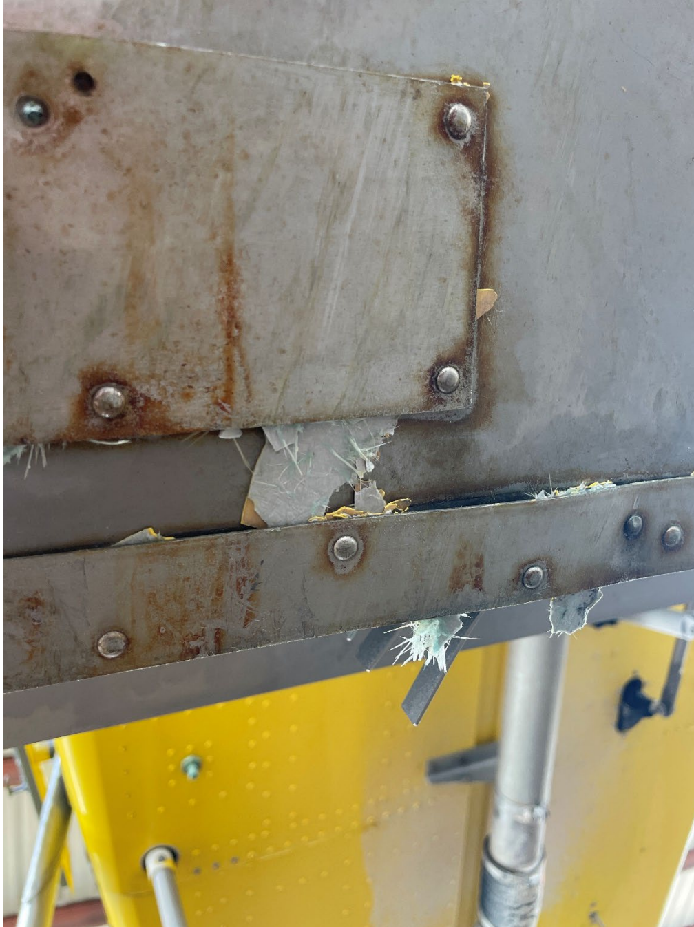
Figure 7. Paint and fiberglass debris located on the underside of N795LA's spreader.
