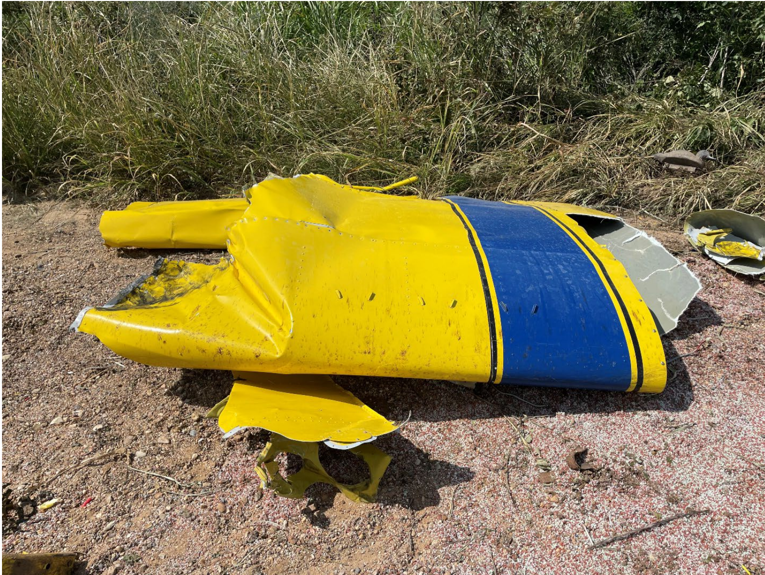
Photograph 9. N6177J Separated outboard left wing
