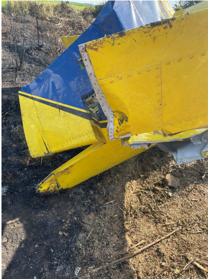
Photograph 11. N6177J Left horizontal stabilizer
