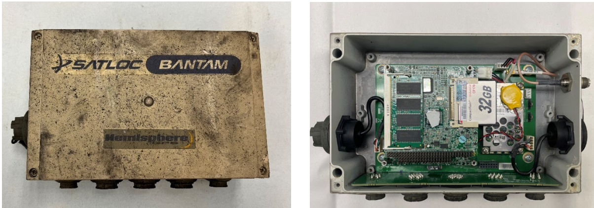
Figure 1. Satloc M3 Bantam device (left) and internal CF card (right).
