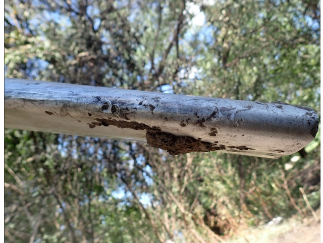
Photograph of threaded fastener impression noted to leading-edge of blade W .
