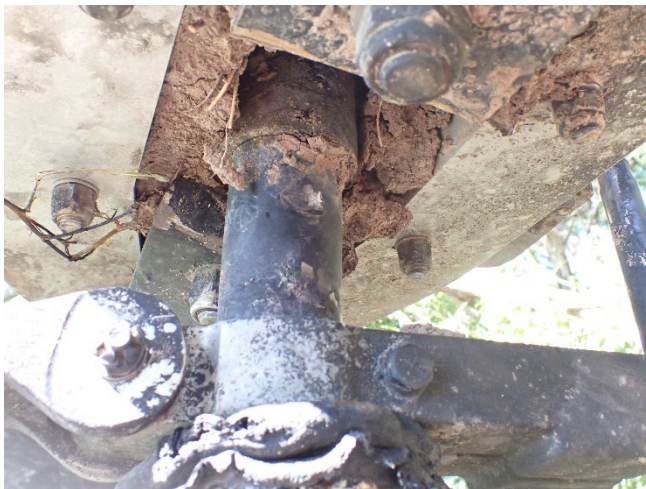
Photograph of main rotor mast impact under blade W .
