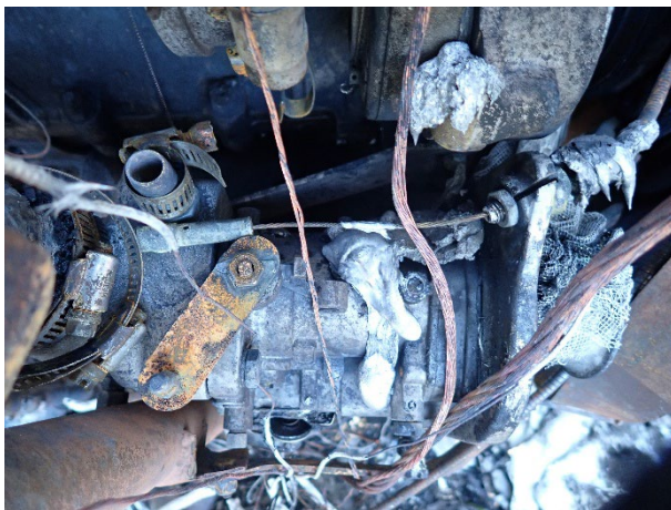
Photograph of snap out ball joint separated from the carburetor.
