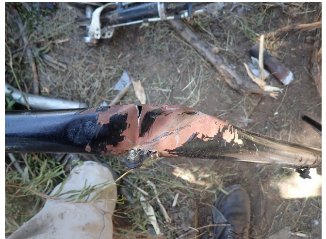
Photograph of separated tailboom structure threaded fastener and blade W impact impression.
