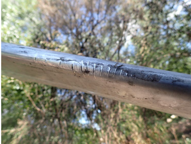
Photograph of tailrotor control cable abrasion noted to leading-edge of blade W .
