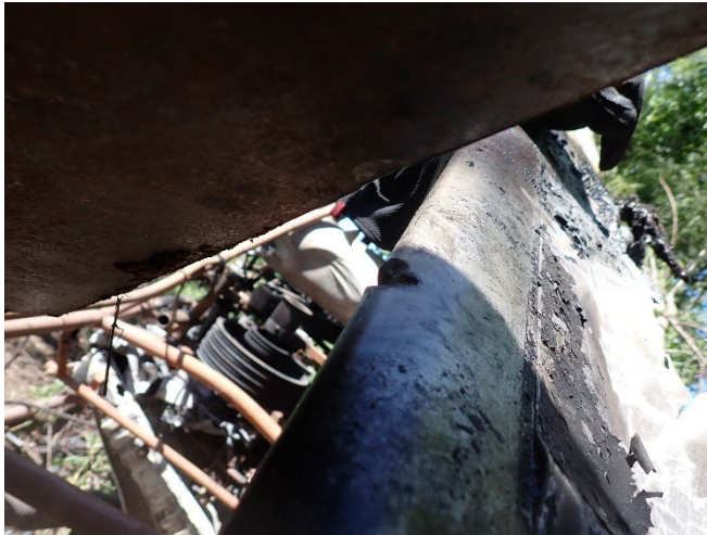
Photograph of ballast weight impact with blade W .
