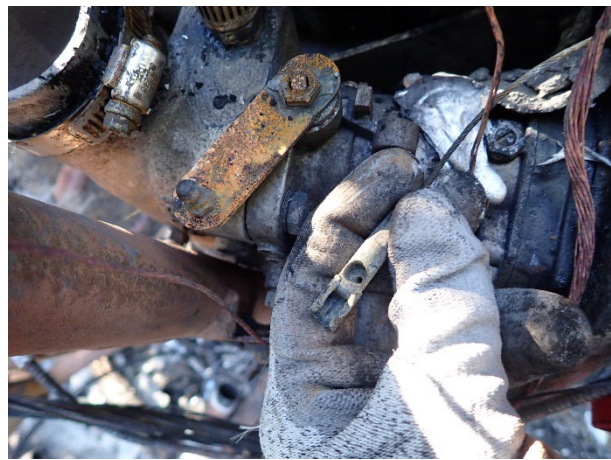
Photograph of ball joint safety not in position.
