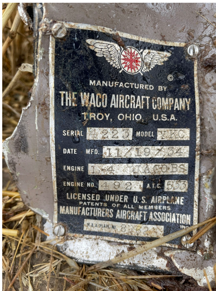
Photograph 6 - Accident Airplane Data Plate
