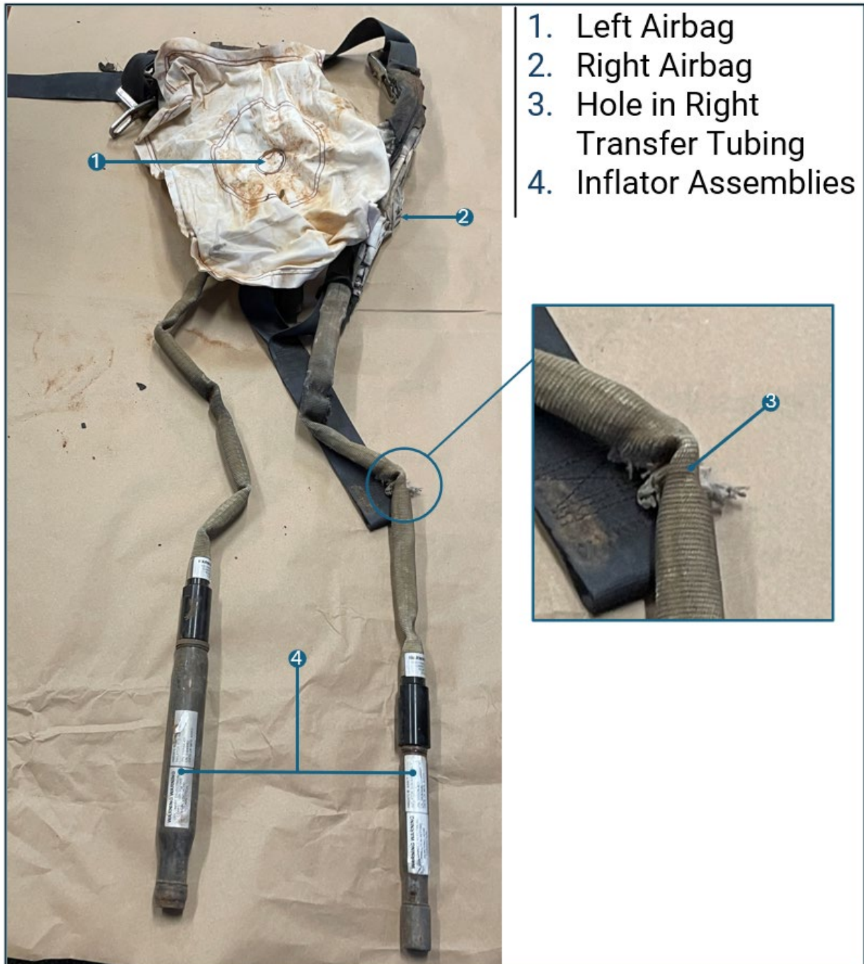
Figure 1 Inflatable restraint system from N8525V (NTSB)
