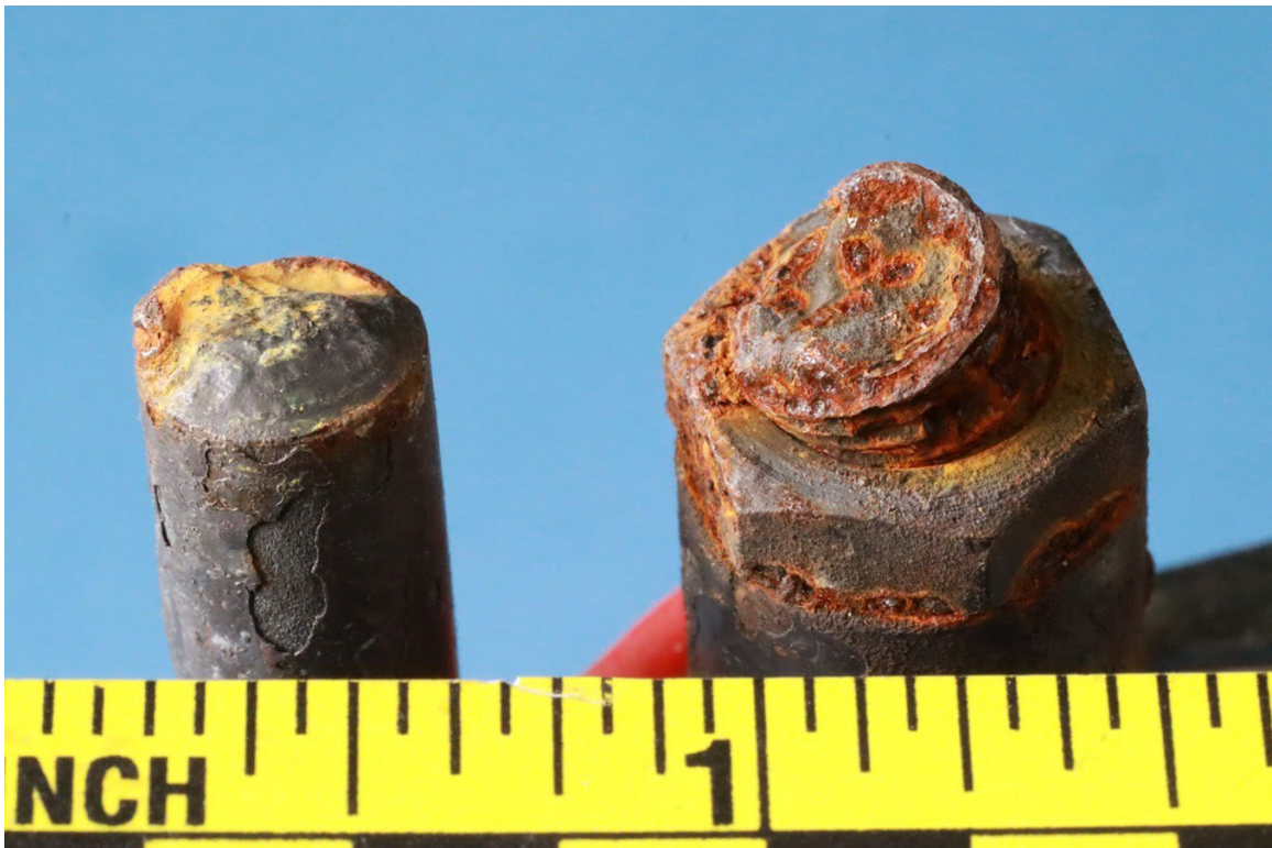
Figure 8. Photograph of the fractured right aileron drooping push rod (shorter rod).
