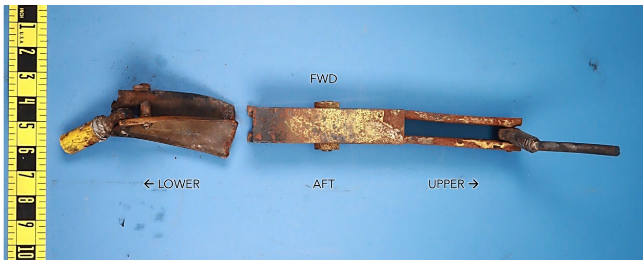
Figure 2. Photograph of the fractured right aileron bellcrank viewed looking outboard.
