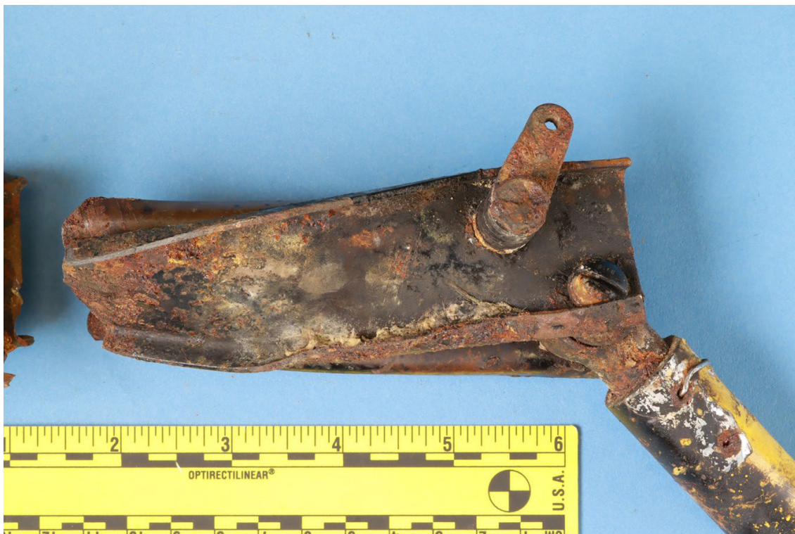
Figure 5. Photograph of the forward side of the lower portion of the fractured right aileron bellcrank showing the bent outboard flange at the lower end.
