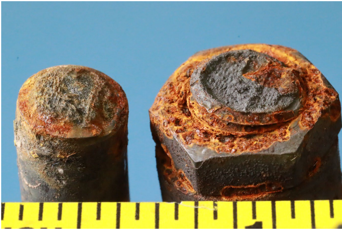
Figure 7. Photograph of the fractured right aileron drooping push rod (longer rod).
