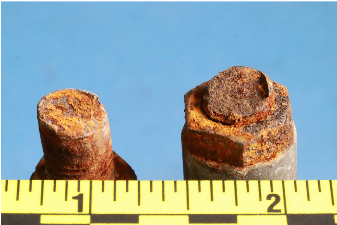
Figure 10. Photograph of the fractured right flap push rod.
