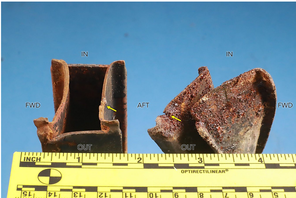
Figure 4. Similar photograph as figure 3 taken from a more oblique angle. A shift in the fracture surface orientation is indicated by yellow arrows.
