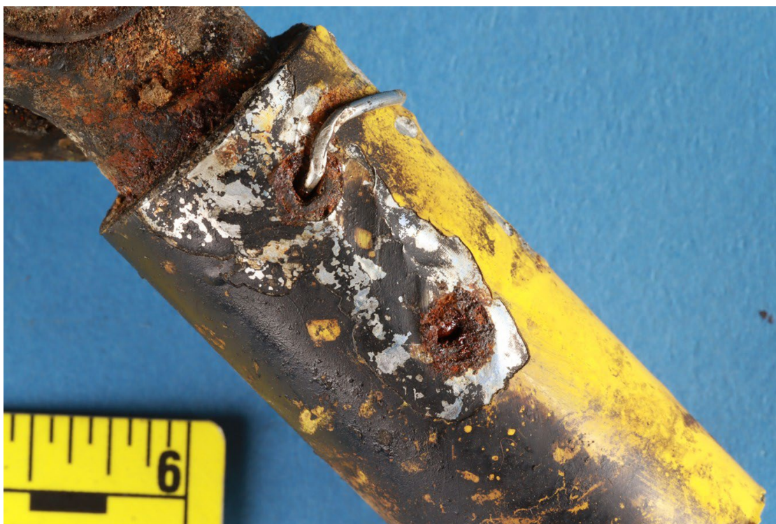
Figure 6. Closer photograph of the forward side of the section of main aileron pushrod retained by the lower portion of the fractured bellcrank showing chipped paint, gouges, and smeared metal.
