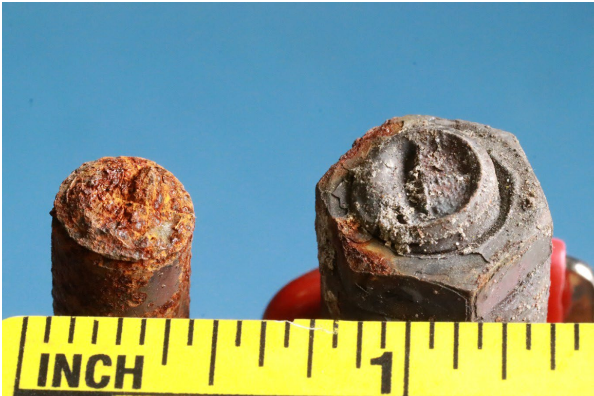
Figure 9. Photograph of the fractured left aileron drooping push rod.
