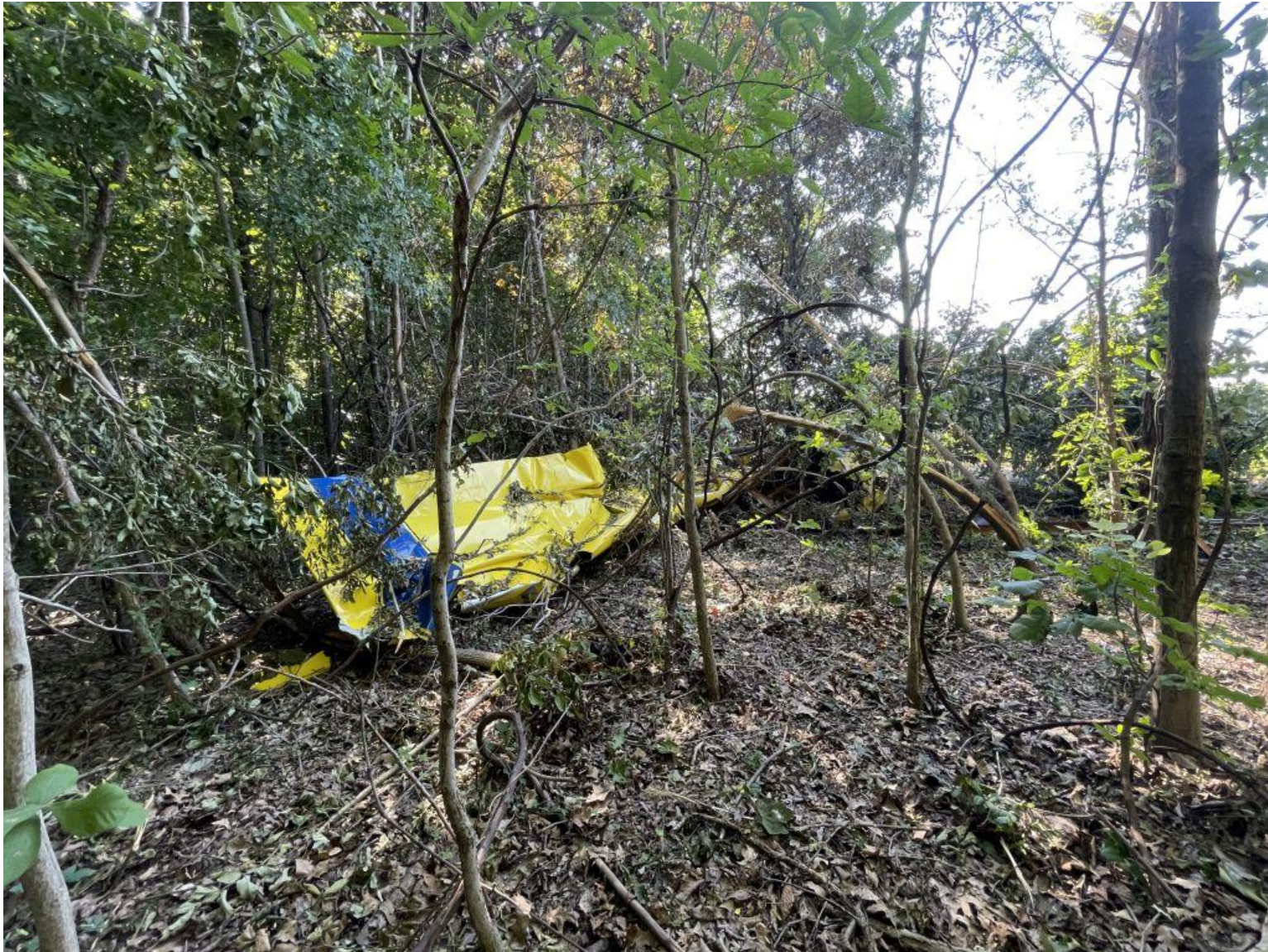
Photograph 4 - Right wing at accident site (NTSB photo)
