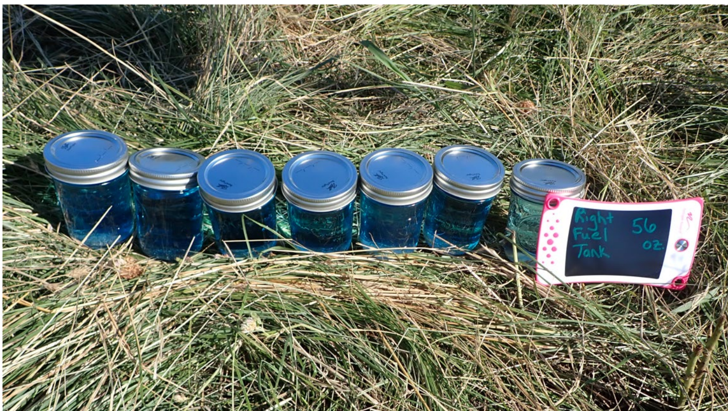
Photograph 10 - Fuel obtained from right wing fuel tank
