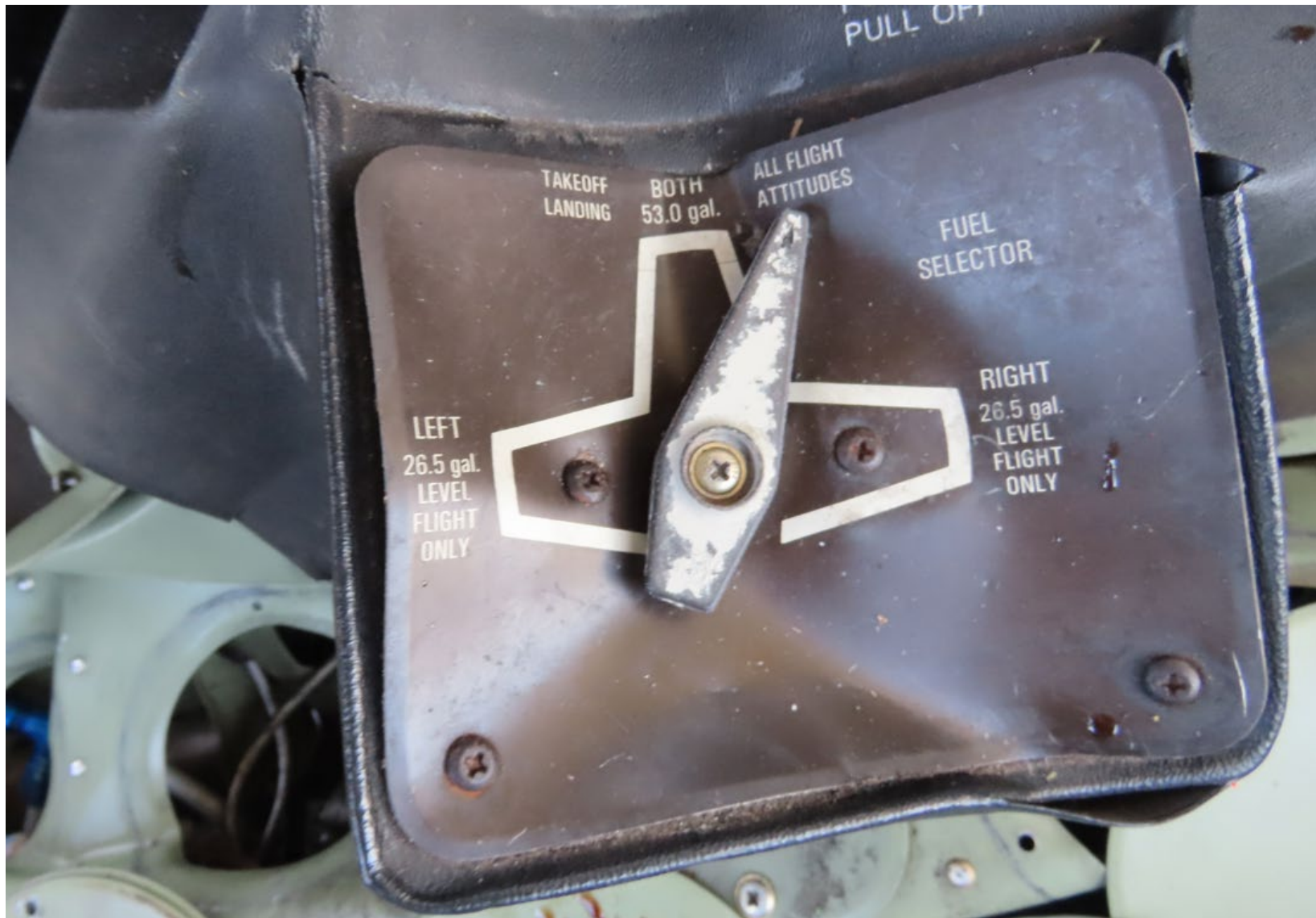
Photograph 6 - Fuel selector valve on both
