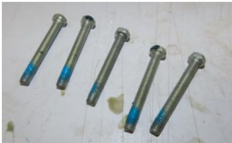
Bottom 5 Screws with Loctite Applied
