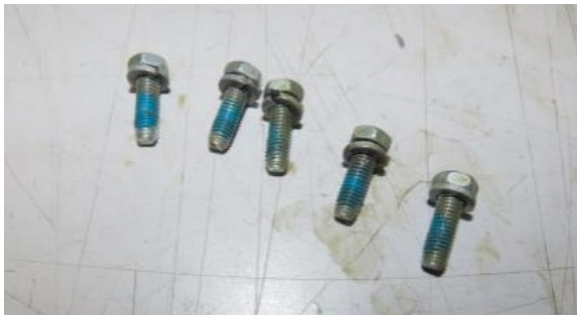
Top 5 Screws with Loctite Applied
