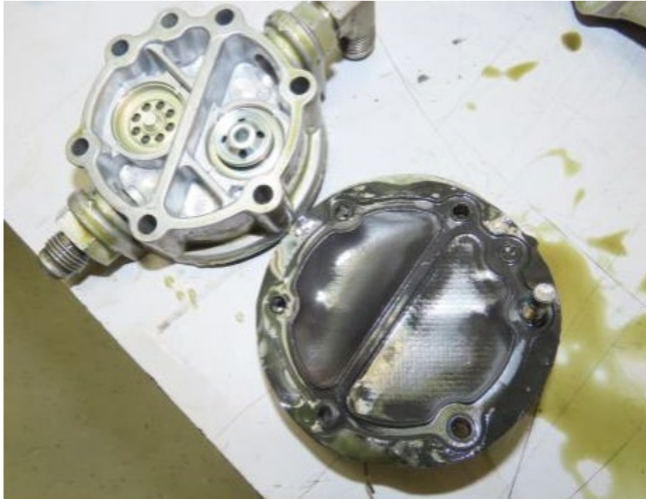
Disassembled Pump Body and Diaphragm
