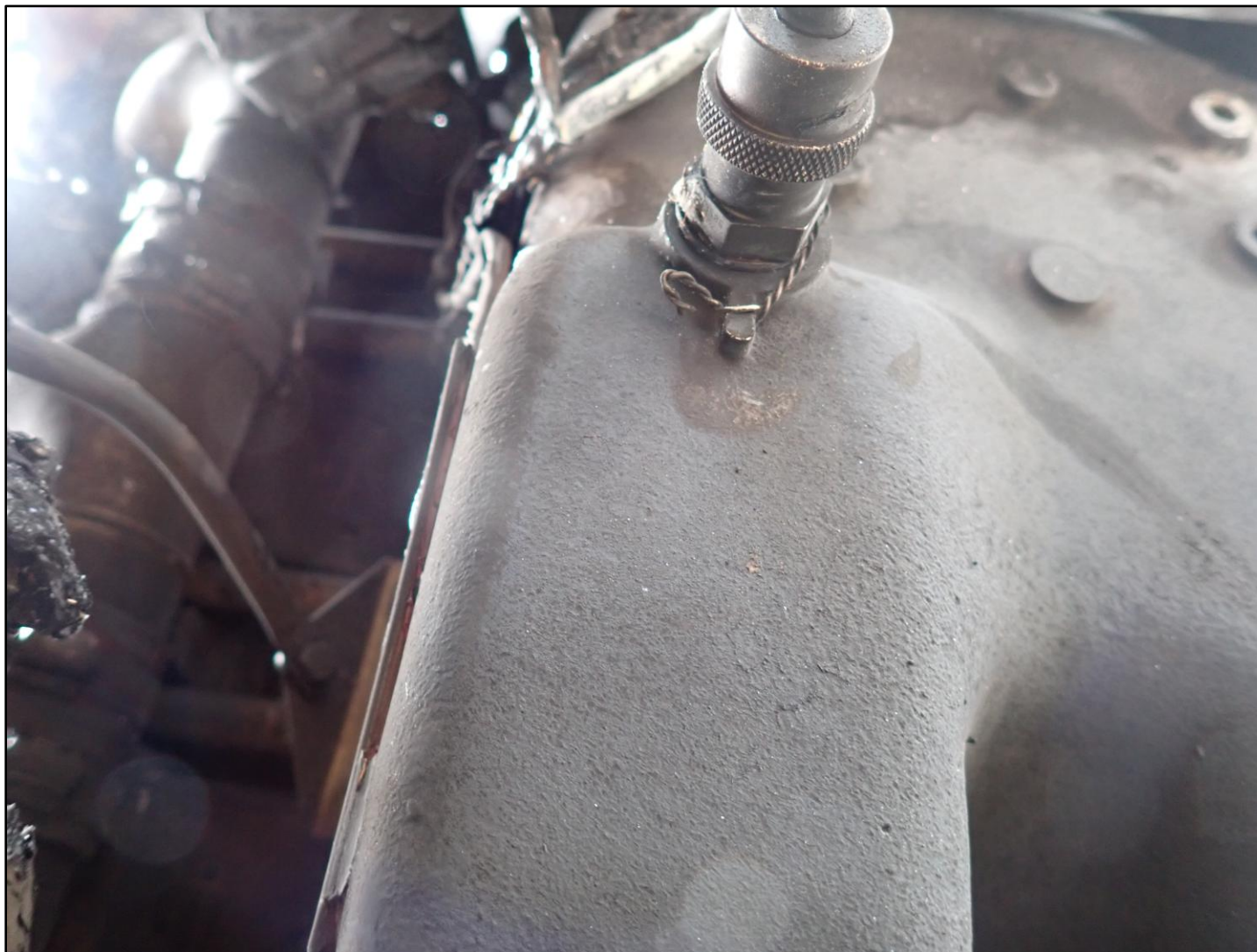
Photograph 5 - Oil quick drain as found at accident site
