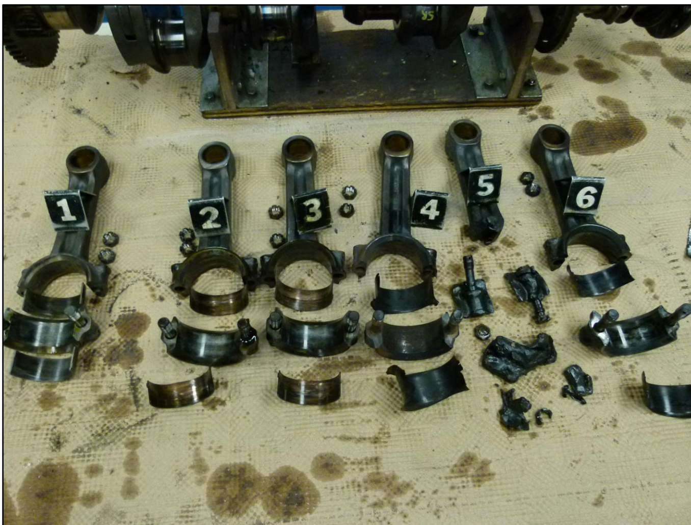
Photograph 6 - Engine examination - connecting rods and bearings (Courtesy of Continental Aerospace Technologies)
