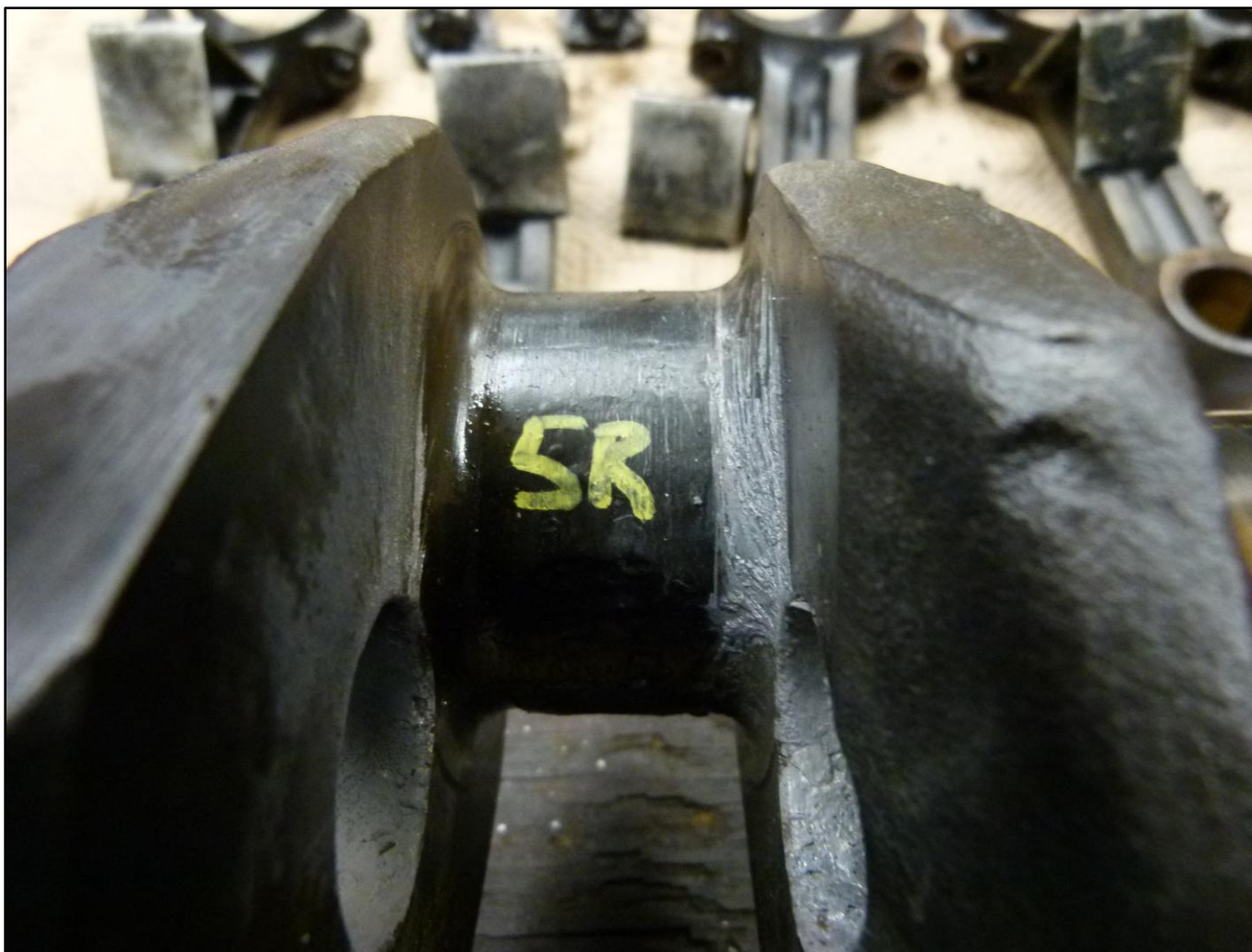
Photograph 7 - Engine examination - No. 5 connecting rod journal (Courtesy of Continental Aerospace Technologies)
