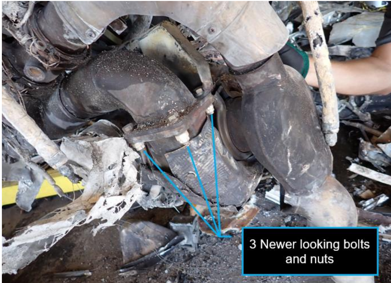
Figure 6. New bolts found during wreckage examination.
