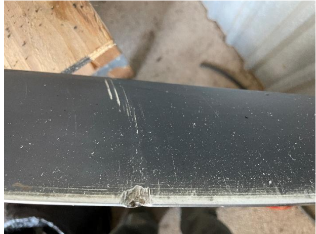
Figure 15. Blade "A" gouge and scrapes
