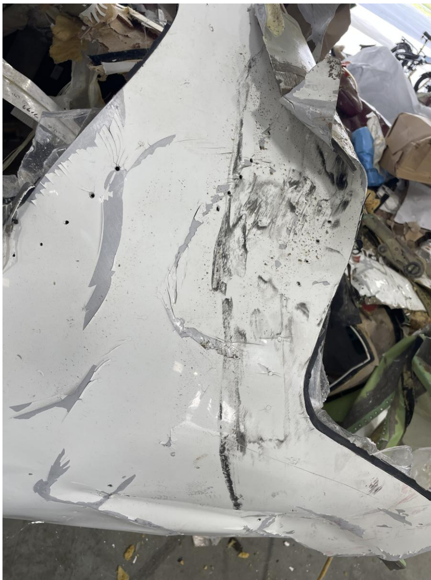
Photograph 2 - Black witness marks right aft fuselage (NTSB Photo)
