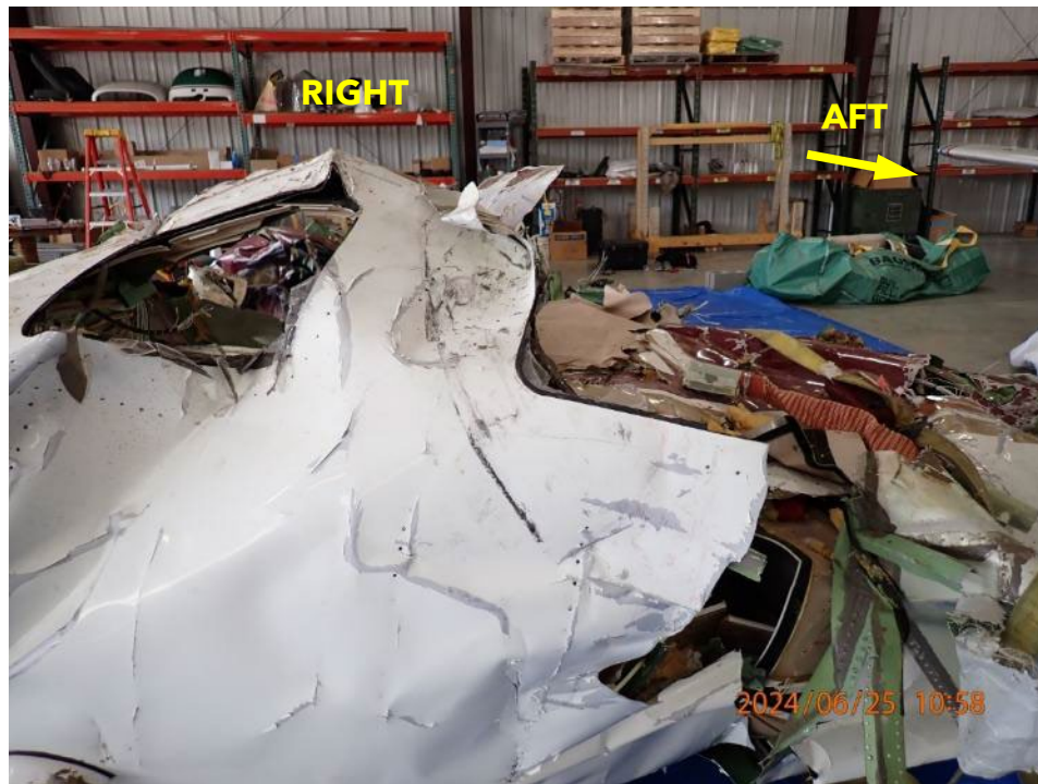
Figure 8. Right side fuselage skin with rubber transfer mark (NTSB photo)
