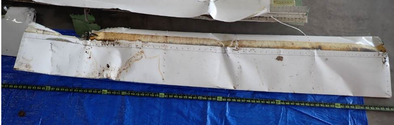
Figure 13. Left flap outboard section (NTSB photo)
