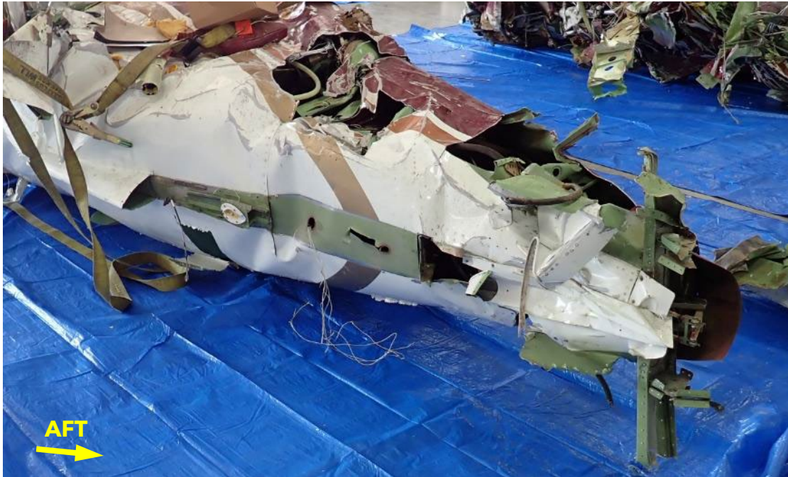
Figure 17. Vertical stabilizer attach locations (NTSB photo)
