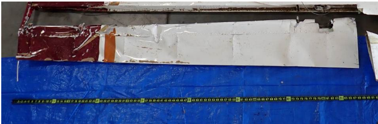
Figure 14. Left Aileron (NTSB photo)
