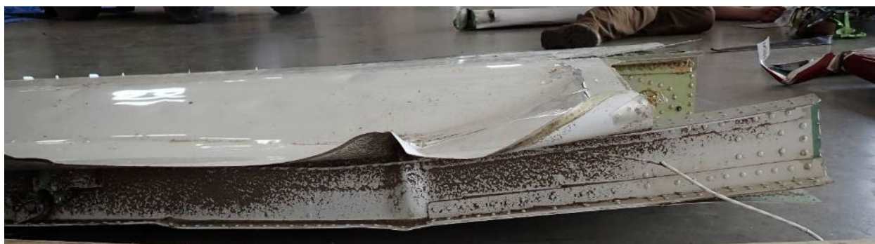
Figure 12. Left wing outboard section spar deformation (NTSB photo)
