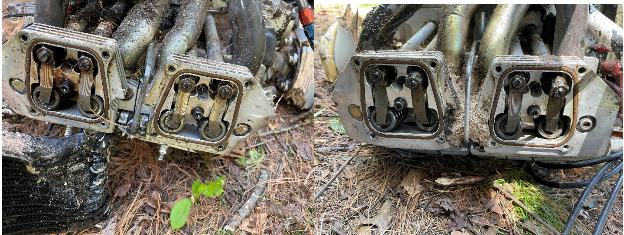
Figure 8/9. Right and left side of the engine with the valve covers removed.
