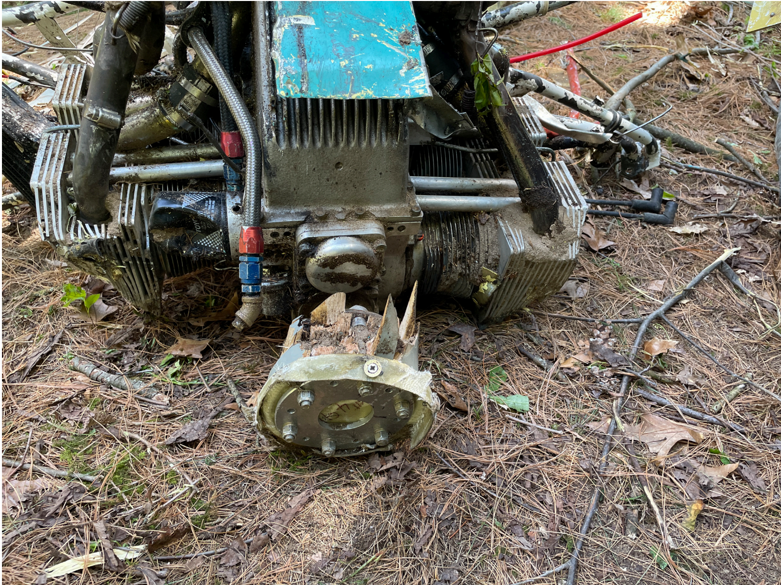
Photograph 8 - Propeller flange (Courtesy of NTSB)
