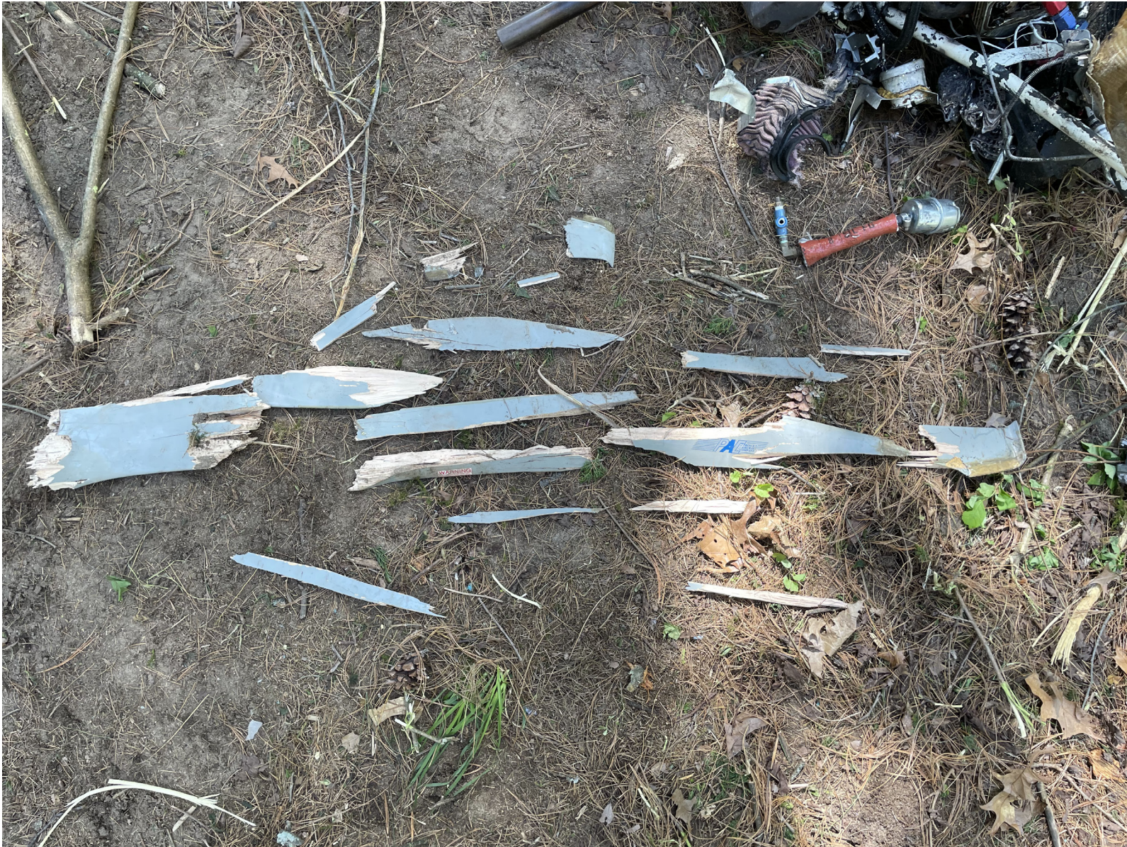
Photograph 9 - Propeller blade pieces (Courtesy of NTSB)
