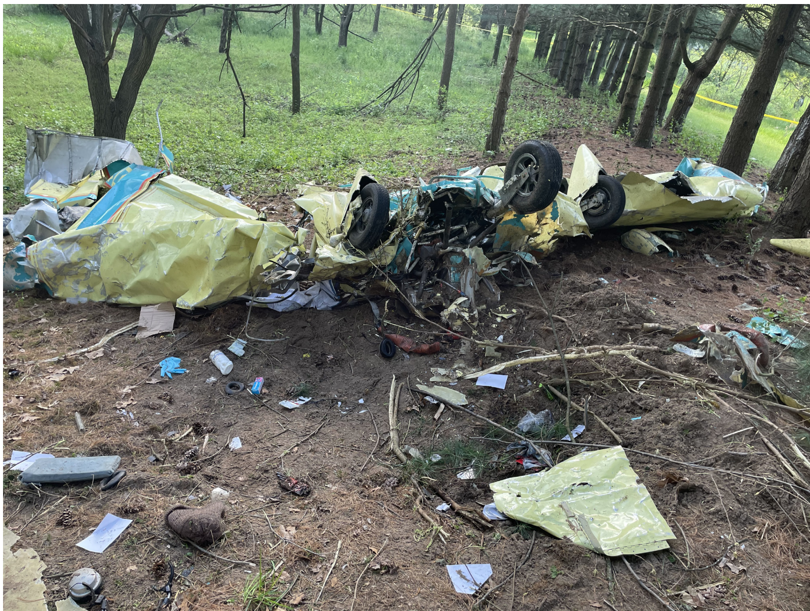
Photograph 7 - Initial impact crater and main wreckage (Courtesy of NTSB)
