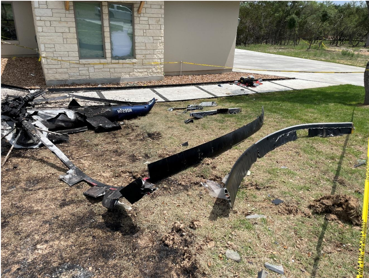
Photograph 9 - View of the main rotor blade remnants during the airframe examination at the accident site
