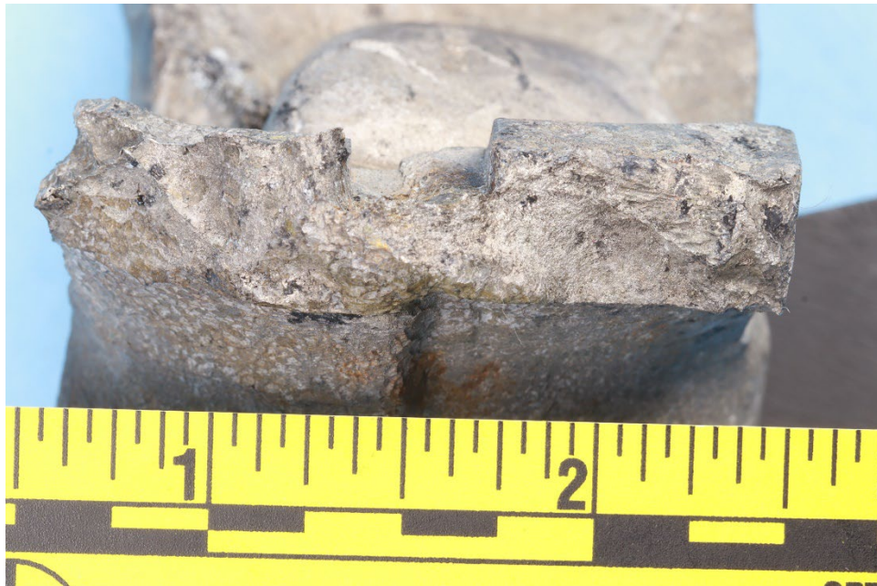
Figure 2. Fracture surface of the arm at the upper side of the photograph in figure 1.
