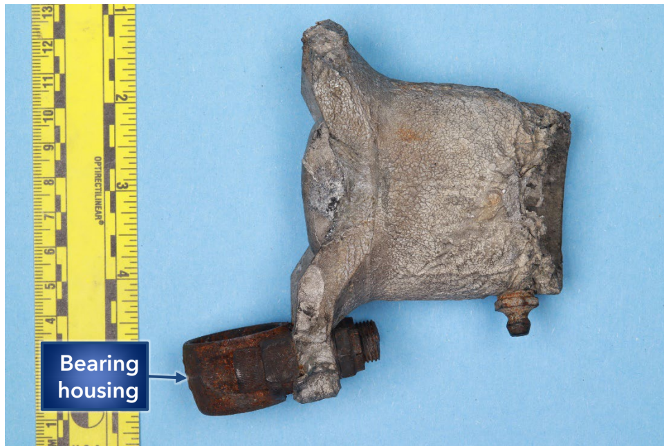
Figure 1. Overall view of the submitted driveshaft universal joint piece.
