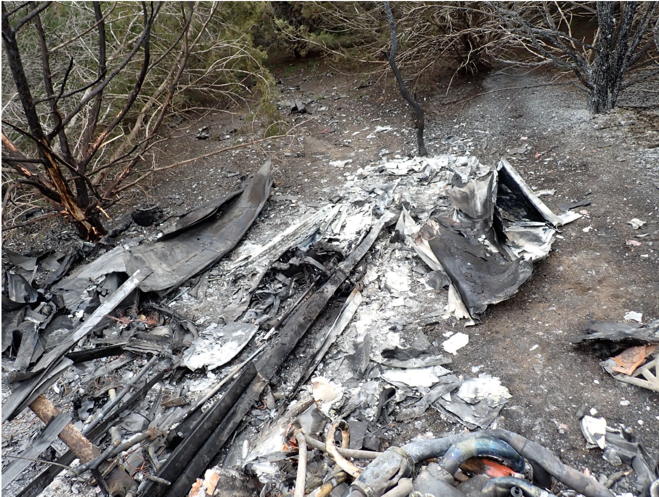
Photograph 2 - Thermal damage noted to left wing.
