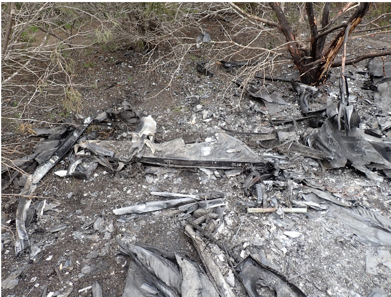
Photograph 4 - Thermal damage noted to empennage.
