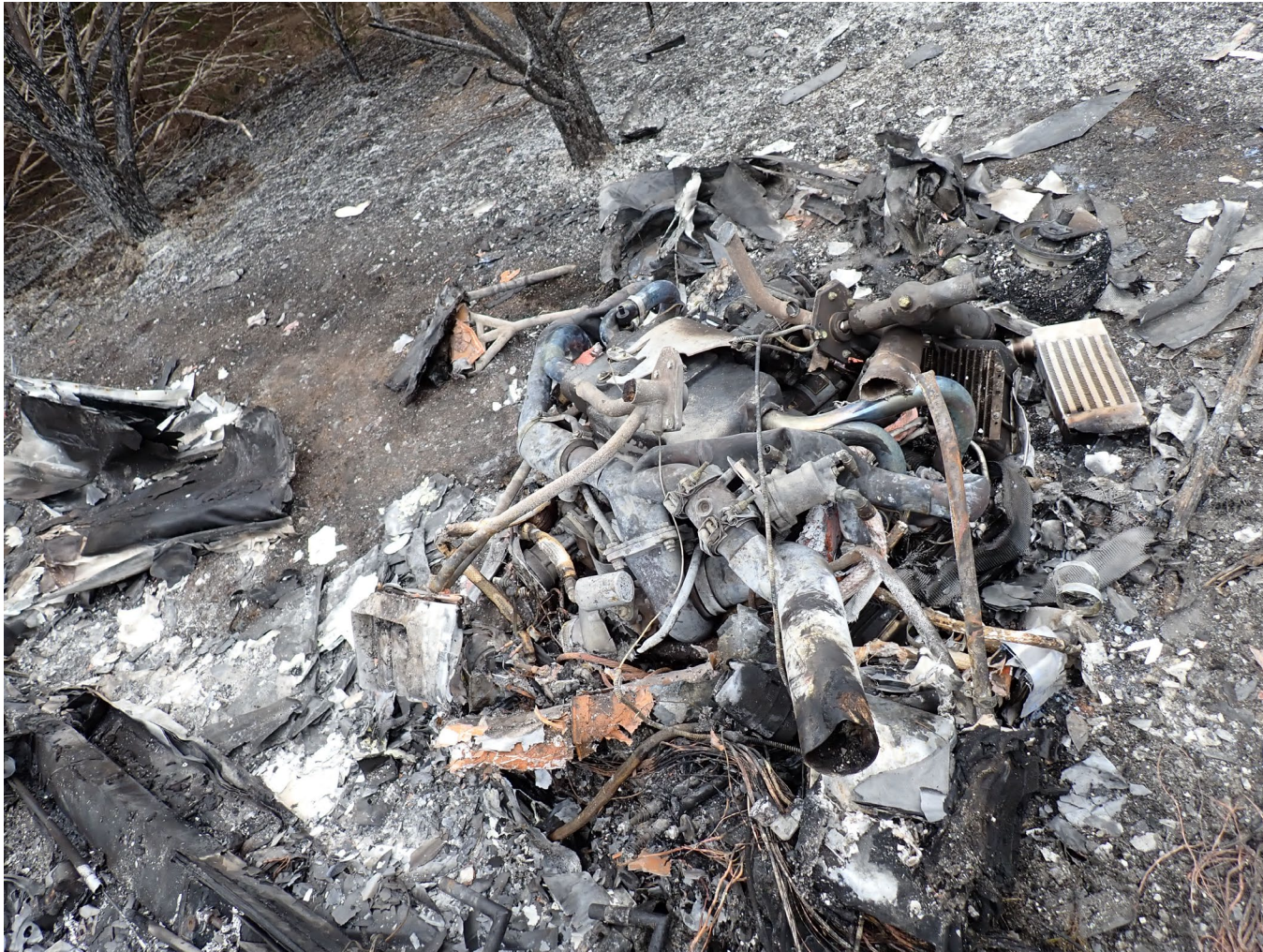
Photograph 5 - Thermal damage noted to engine.
