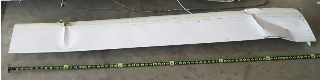
Figure 19. Left flap outboard section (NTSB photo)
