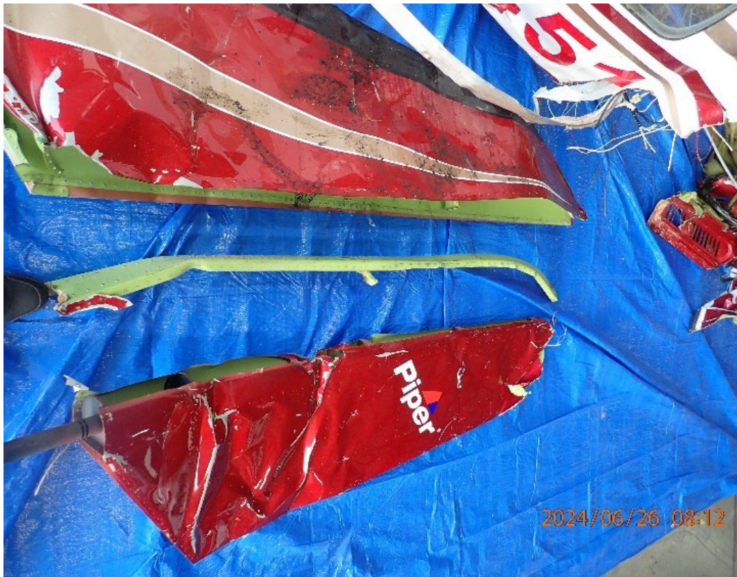
Figure 24. Vertical stabilizer, aft spar and rudder (NTSB photo)
