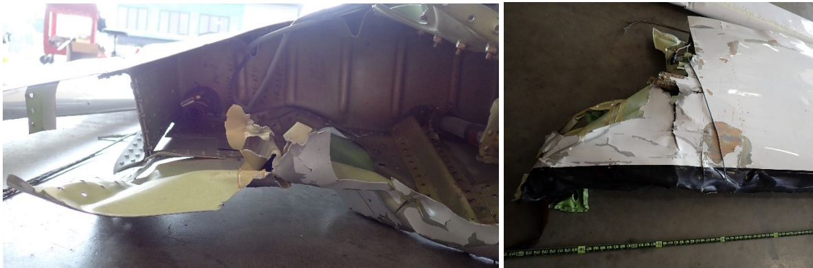
Figure 16. Left wing outboard section aft spar (left) and leading edge (right) (NTSB photos)
