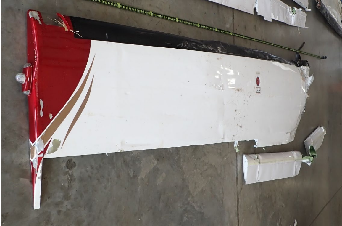
Figure 15. Left wing outboard section. (NTSB photo)
