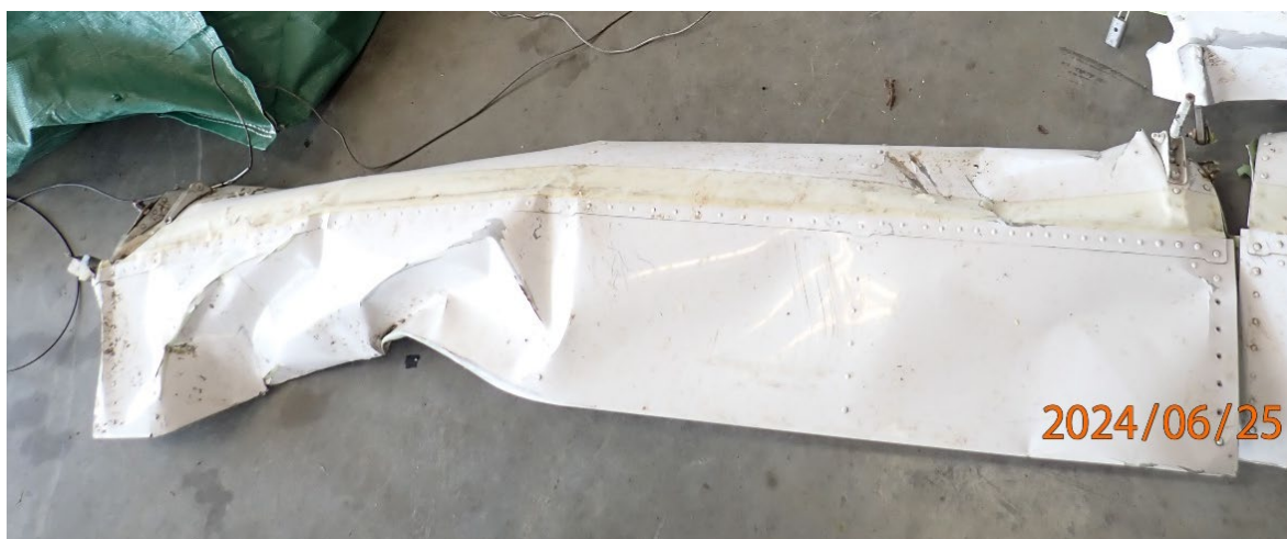
Figure 11. Right flap inboard section (NTSB photo)
