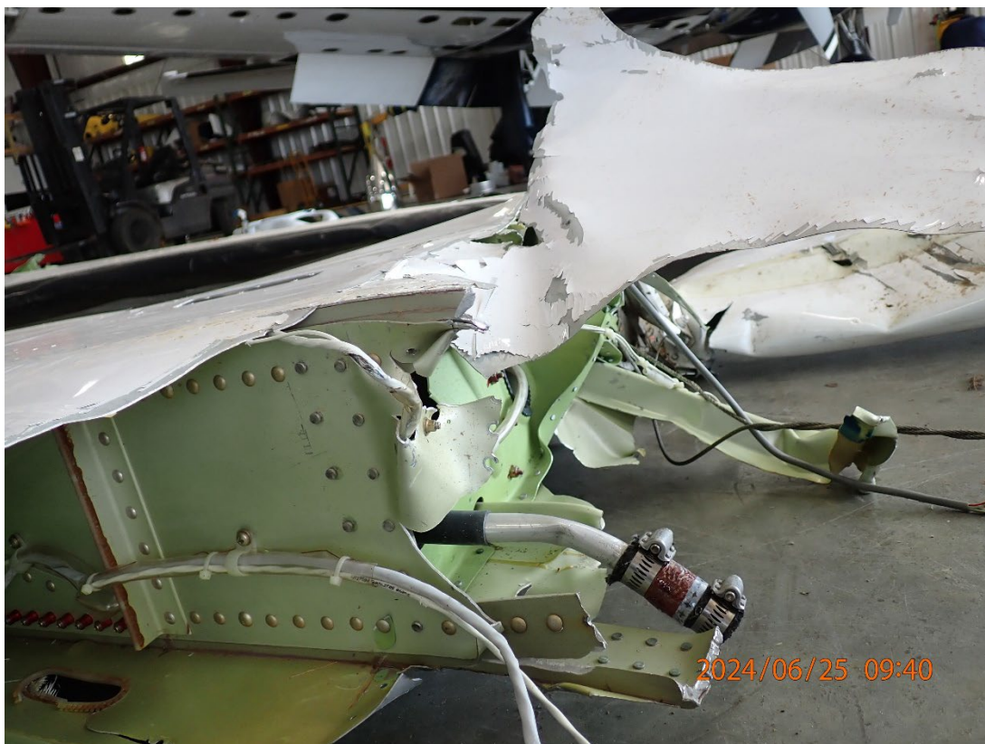
Figure 10. Right wing outboard section main spar fracture (NTSB photo)
