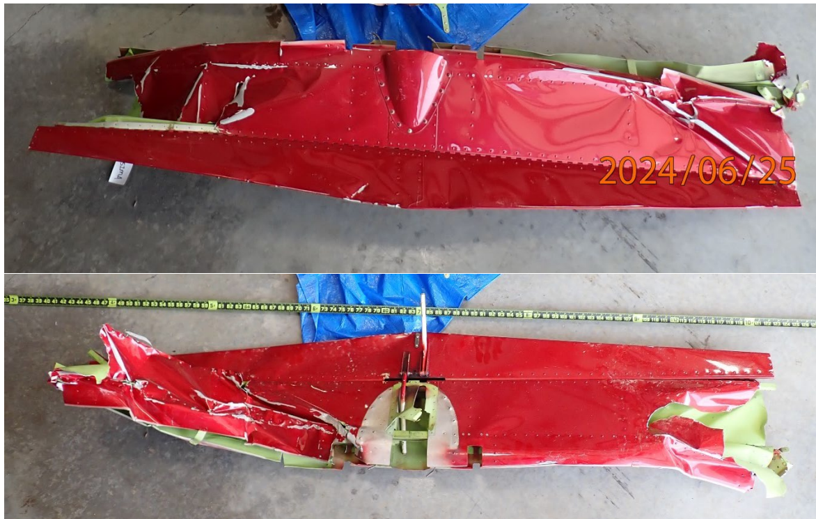
Figure 22. Elevator top side (above) bottom side (below) (NTSB photo)
