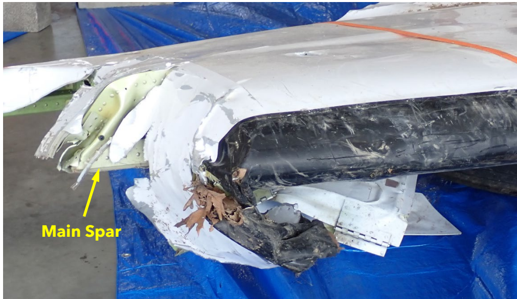
Figure 7. Right wing inboard section fractured leading edge and main spar (NTSB photo)
