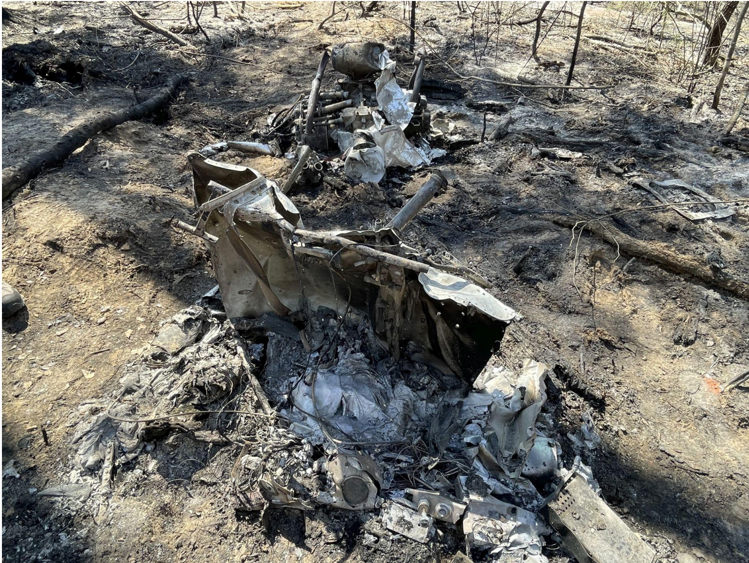
Photograph 7 - Instrument panel / firewall / engine (NTSB photo)
