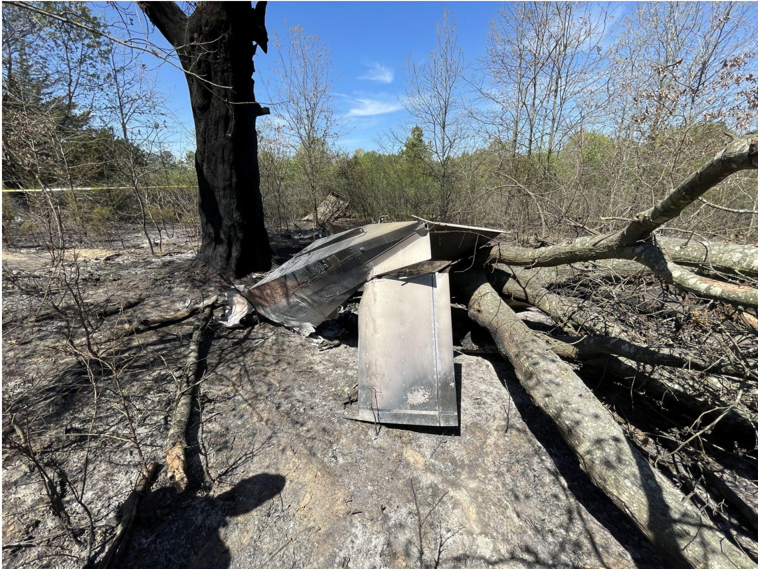
Photograph 3 - Aft fuselage / empennage (NTSB photo)
