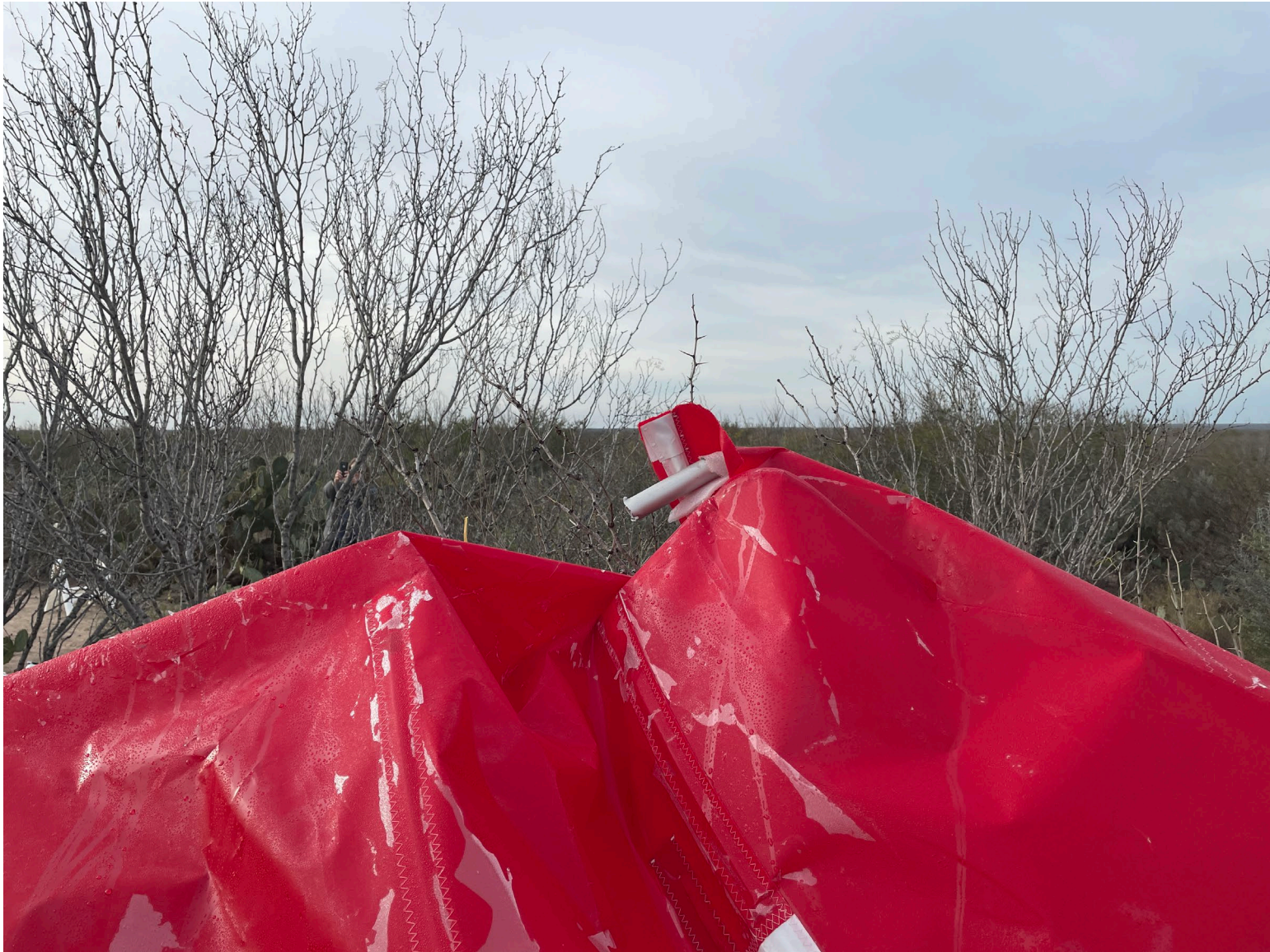
Photograph 4 - Tower Impact Point on Left Wing Tip Leading Edge
