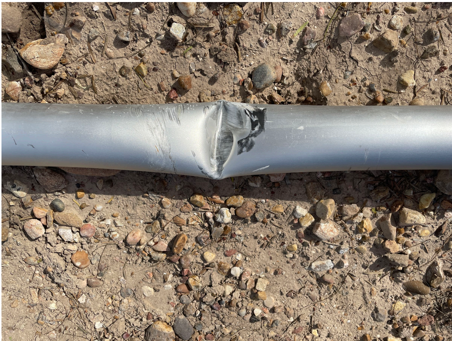
Photograph 3 - Wire Strike Witness Mark Aft Spar
