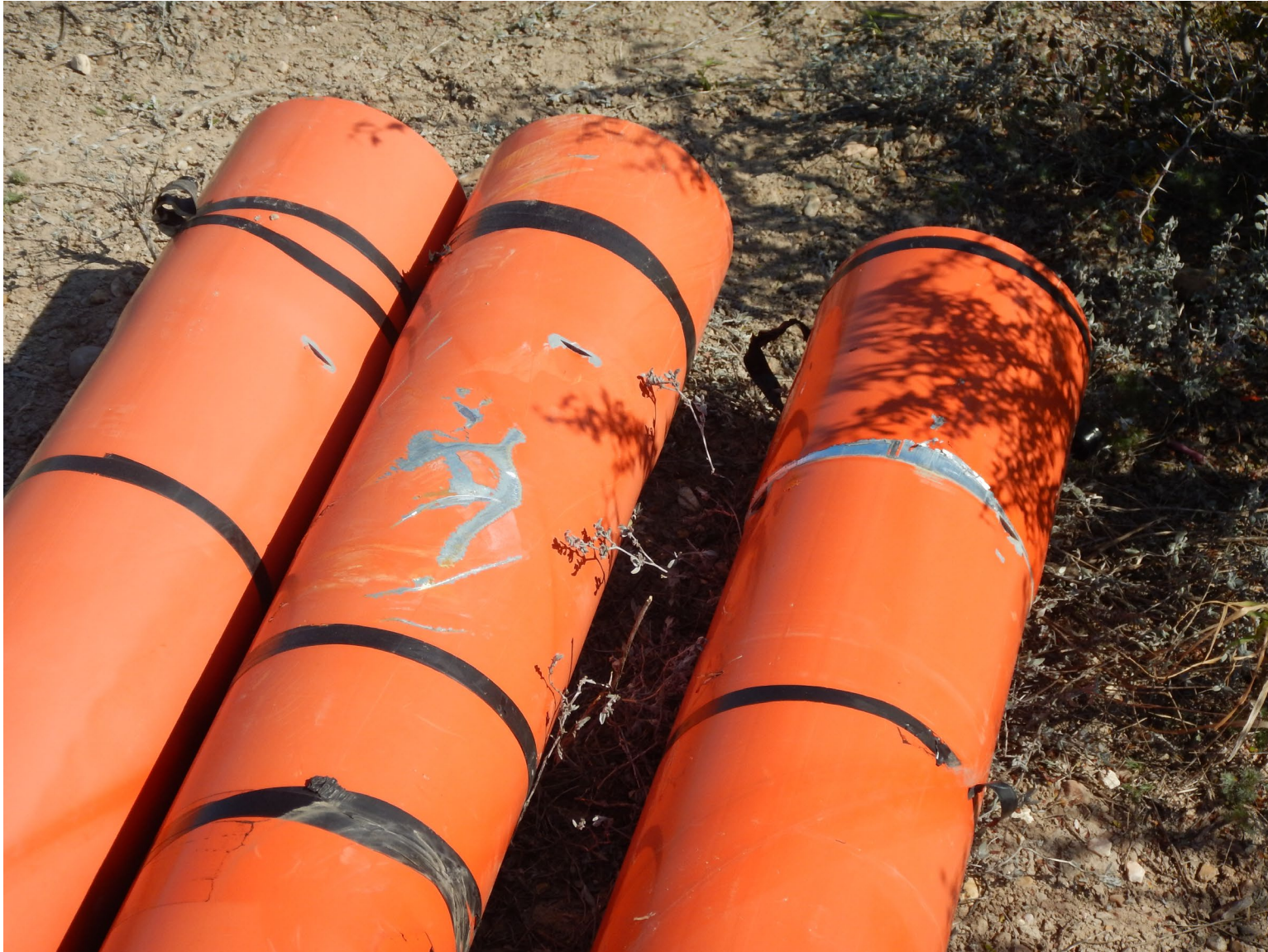
Photograph 5 - Left Wing Impact Witness Marks on Tower Mast
