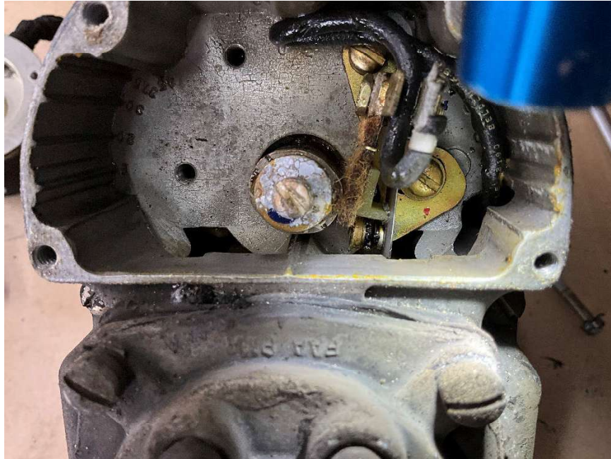
Figure 3. Right Magento contacts prior to cleaning.
