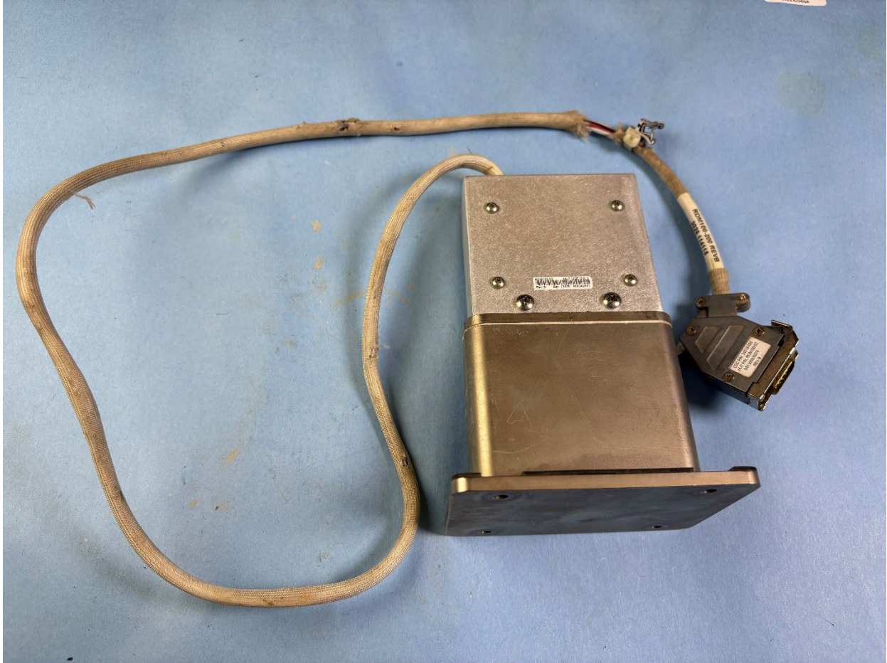
Figure 1. Undamaged RDM-100 as received by the NTSB vehicle recorder laboratory.
