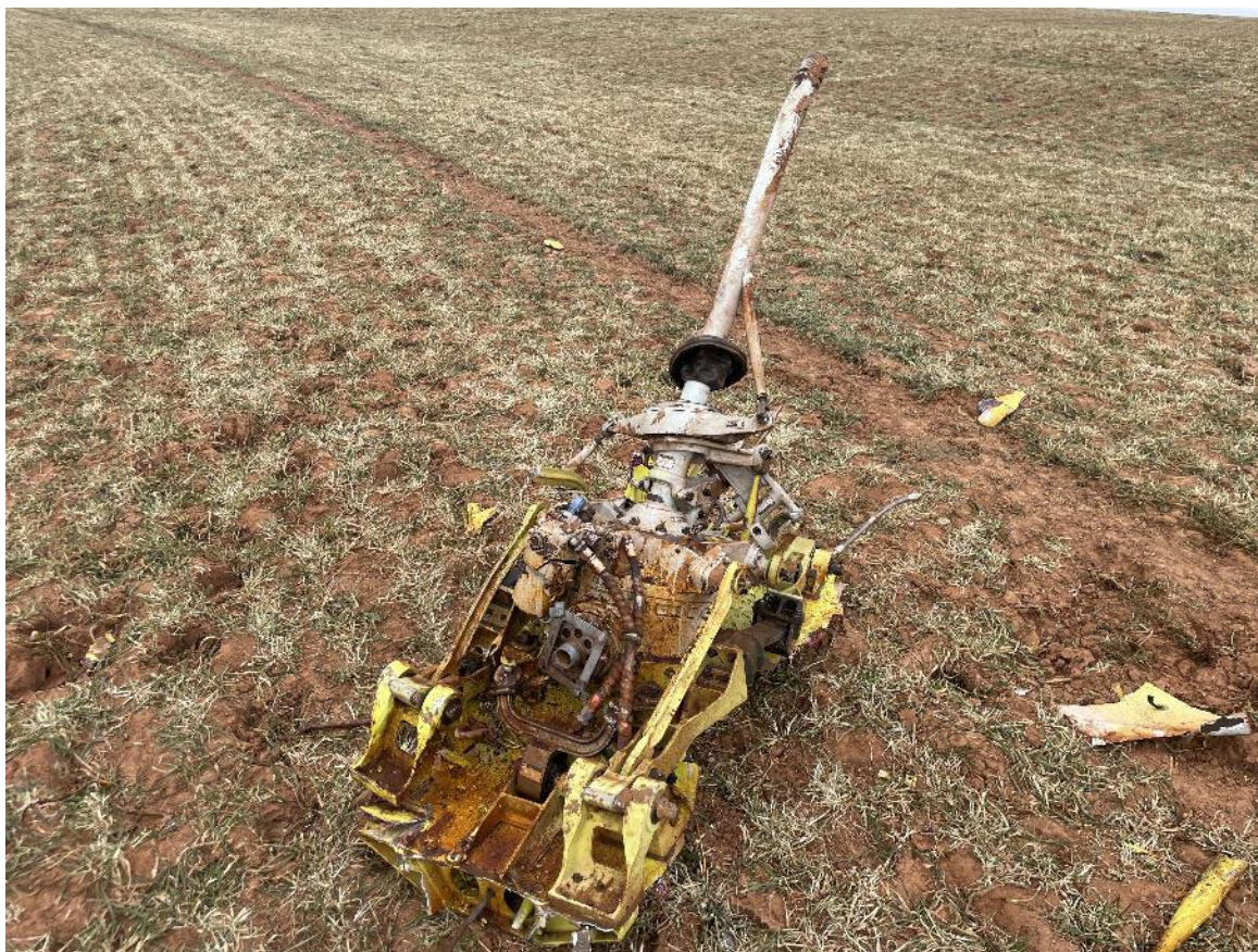
Photograph 2 - Main Rotor Mast & Transmission
