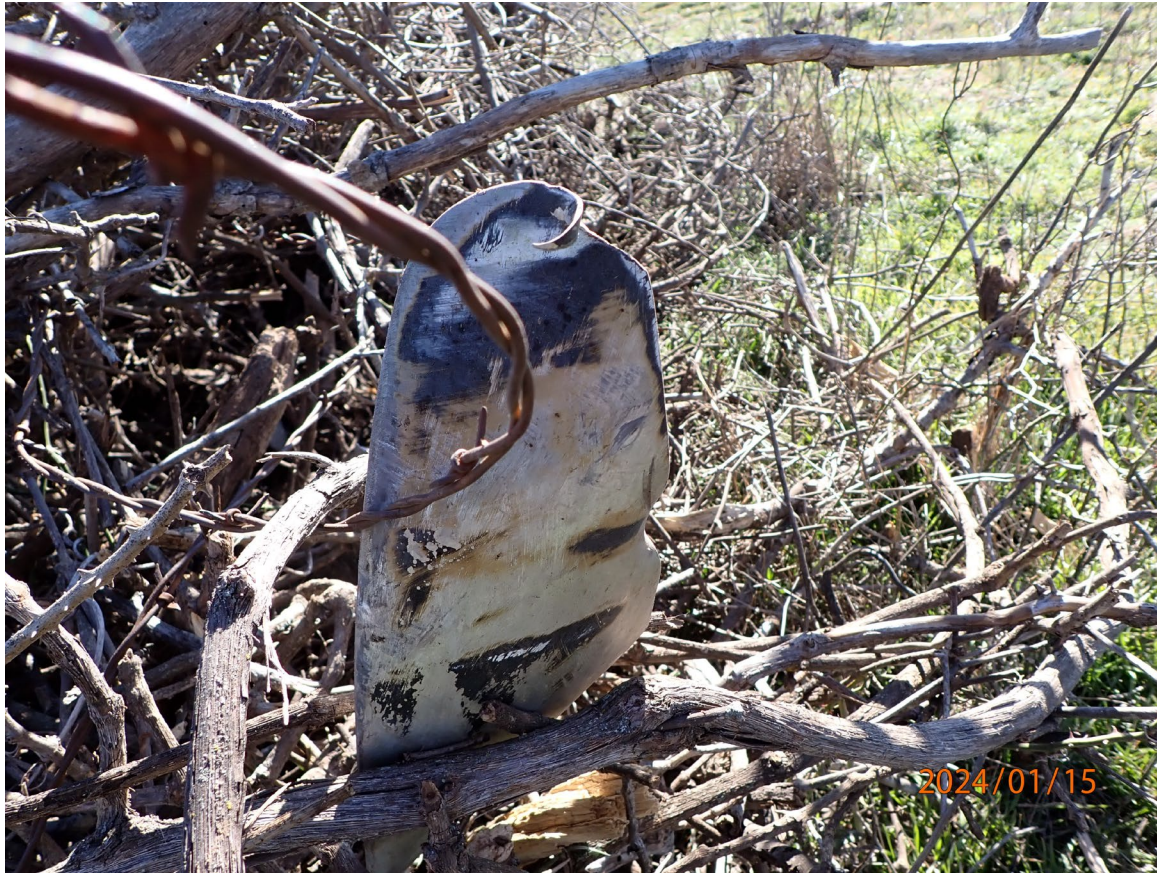
Photograph 3 - Right propeller blade in bush
