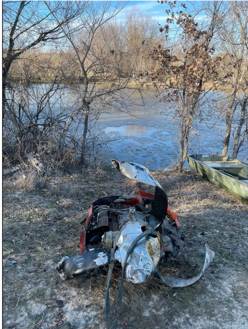
Photograph 8 - Left engine and left propeller
