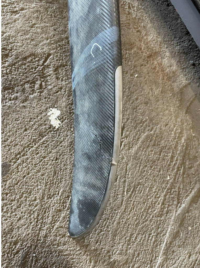
Figure 27. Propeller Blade C Fracture.
