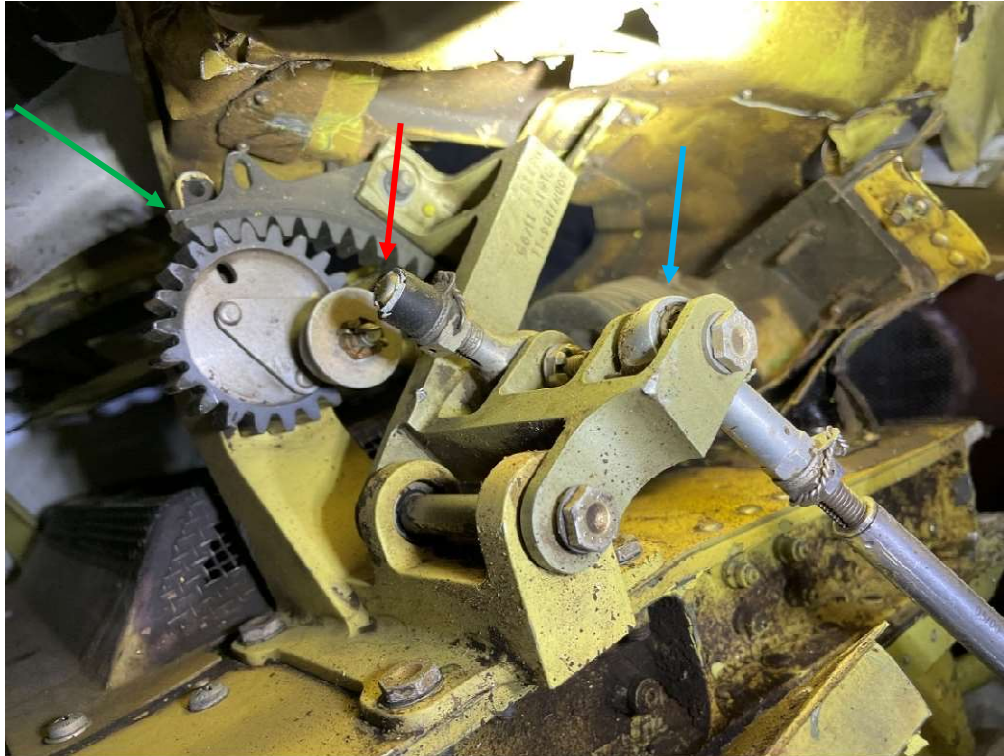
Figure 8. The splitter assembly. The green arrow points to the pitch change control gear. The red arrow points to the aft rod end of the longitudinal control tube. The blue arrow points to the forward cable connection to the splitter assembly.
