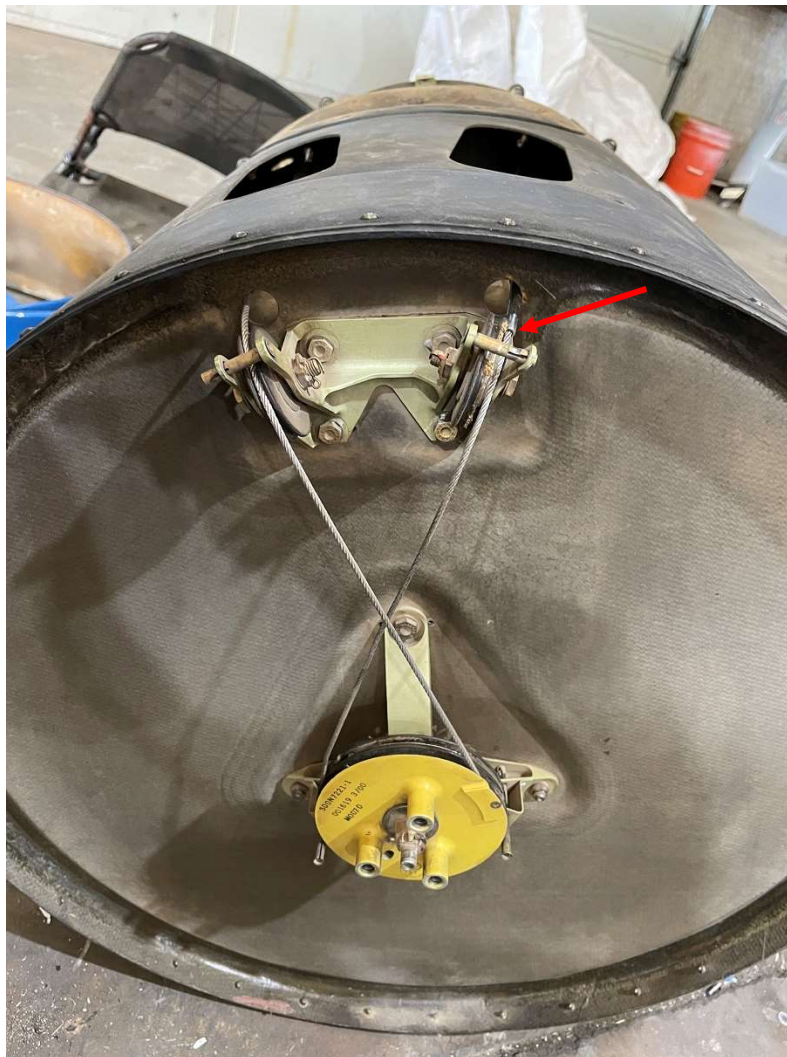
Figure 9. The pulley cable installation for the drum assembly, after removal of the drum (aft looking forward). The yellow-colored pulley on the lower portion of the image is the drum assembly pulley. The red arrow points to the damaged idler pulley.
