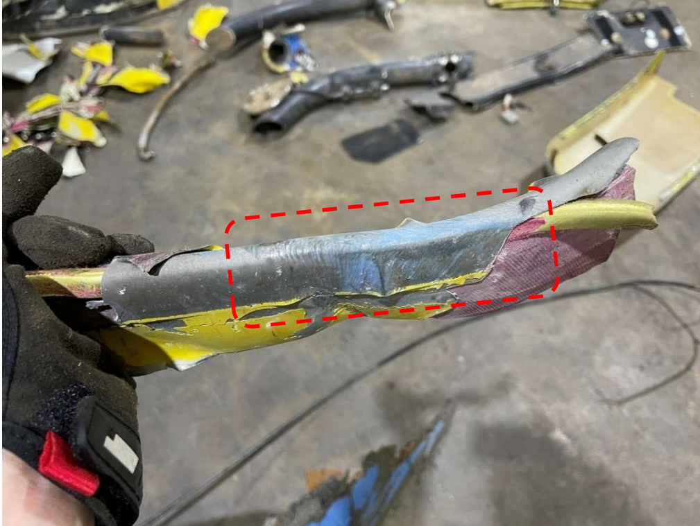
Figure 5. Paint transfer observed on the leading edge of main rotor blade fragments.
