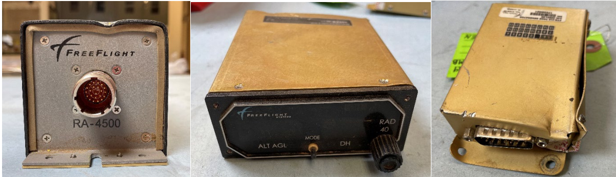
Figure 2. FreeFlight Systems avionics. RA4500 (left), RAD-40 (center), and FTG-410 (right).
