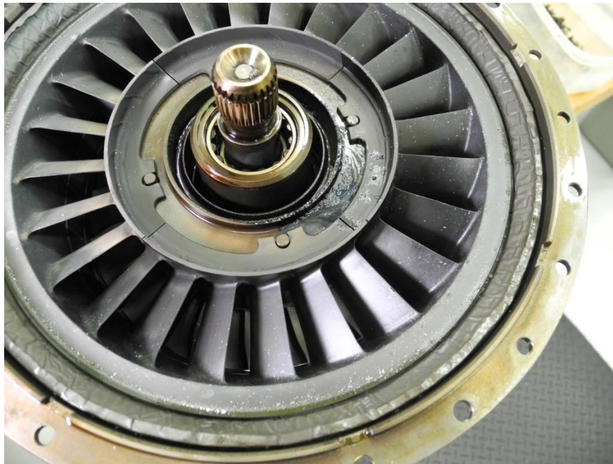
Photo 24 - 3 rd Stage Nozzle - Undamaged
