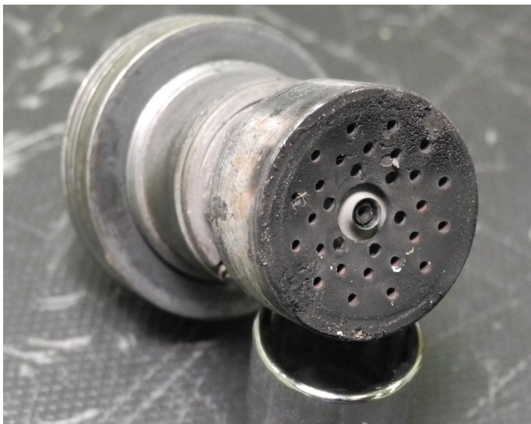
Photo 20 - Fuel Nozzle - Undamaged
