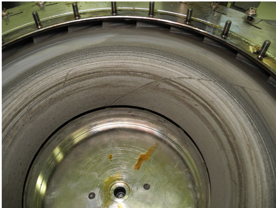
Photo 13 - Impeller Shroud - Scored
