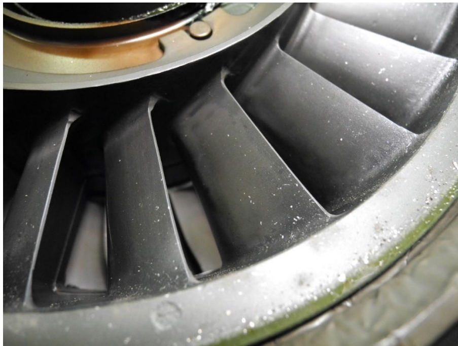
Photo 25 - 3 rd Stage Nozzle - Metal Spray Details
