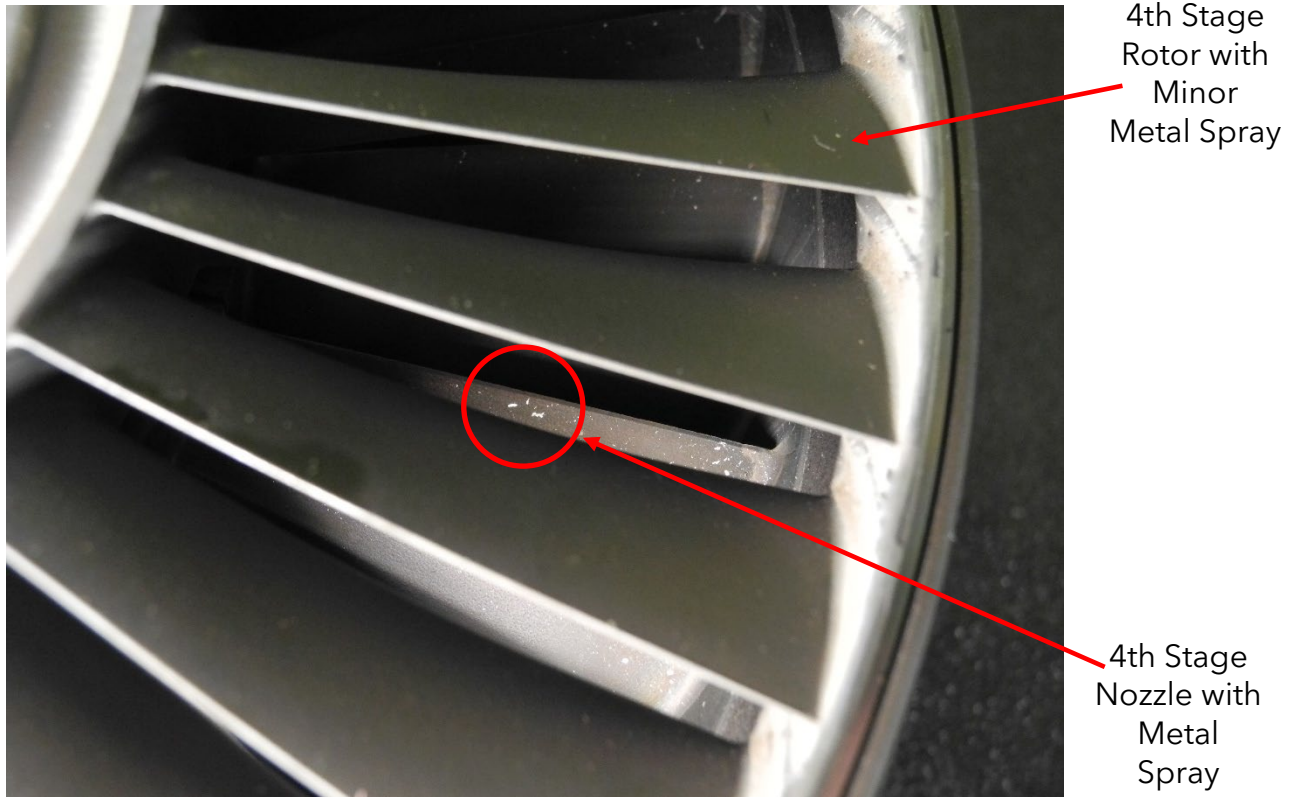
Photo 26 - 4 th Stage Rotor & Nozzle - Metal Spray
