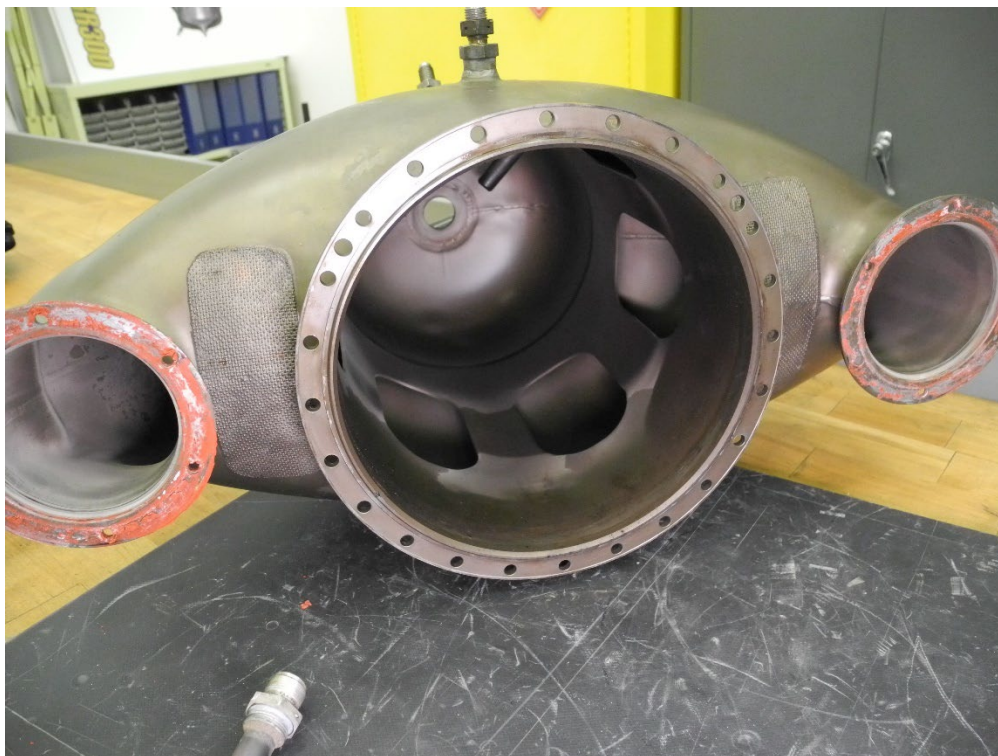
Photo 18 - OCC Internal View - Undamaged
