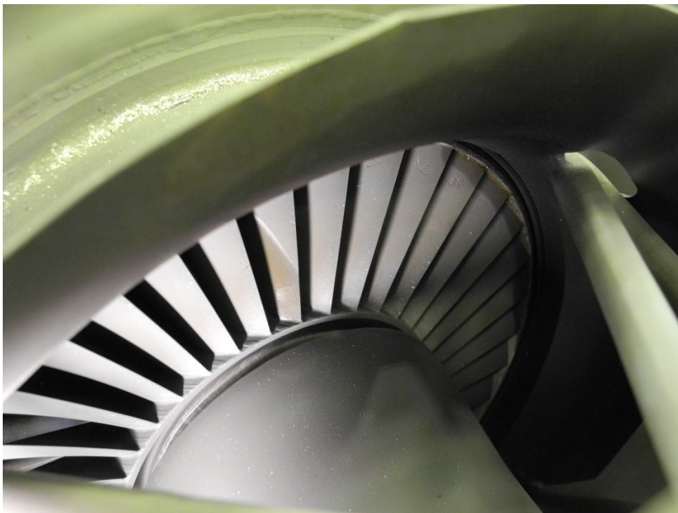
Photo 6 - 4 th Stage Turbine Wheel - Undamaged
