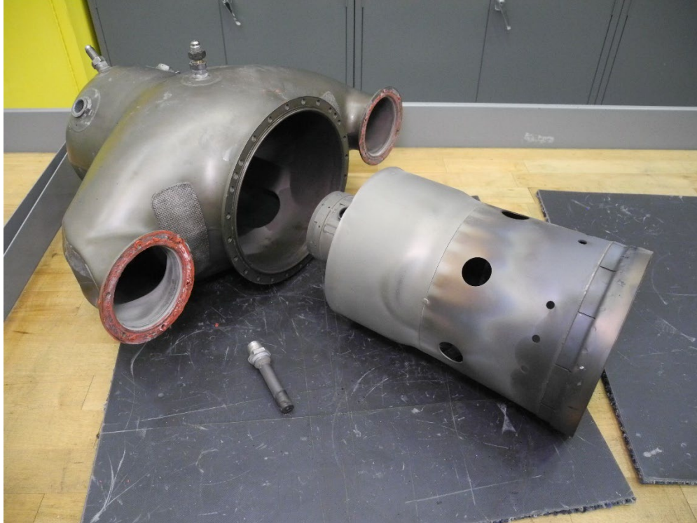
Photo 17 - OCC and Combustor Liner - Undamaged
