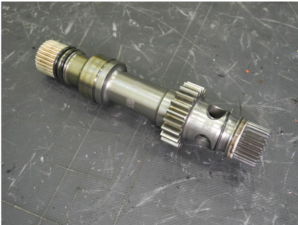
Photo 15 - Spur Adapter Gearshaft - Undamaged
