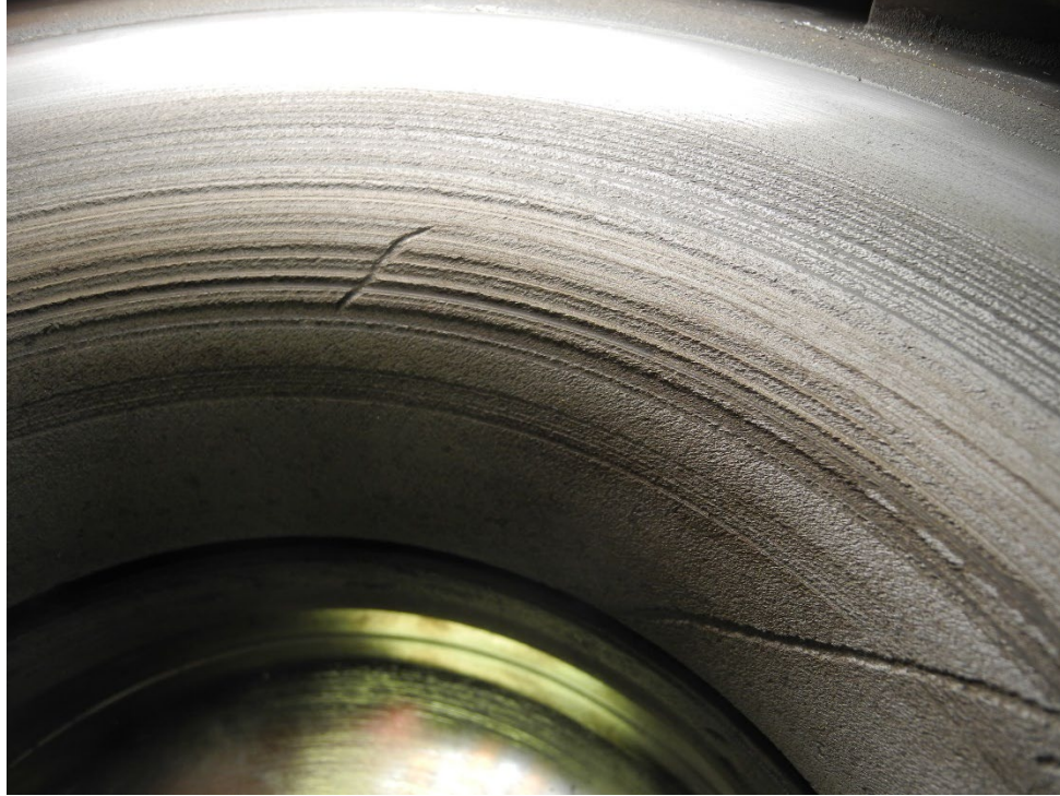
Photo 14 - Impeller Shroud - Scoring Details
