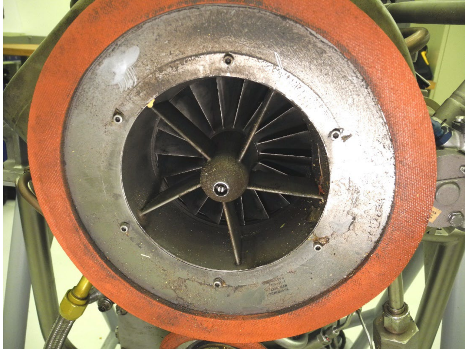
Photo 7 - Compressor Impeller Inlet - Clean
