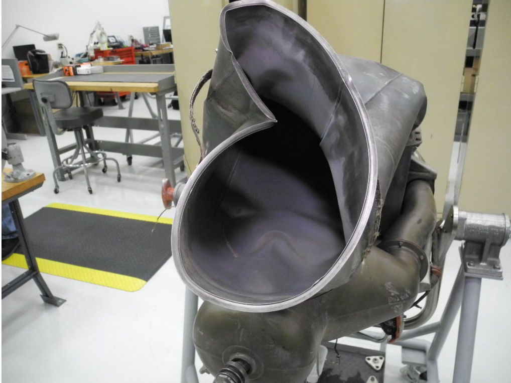
Photo 3 - Airframe Exhaust Duct - Internal Surfaces Dry
