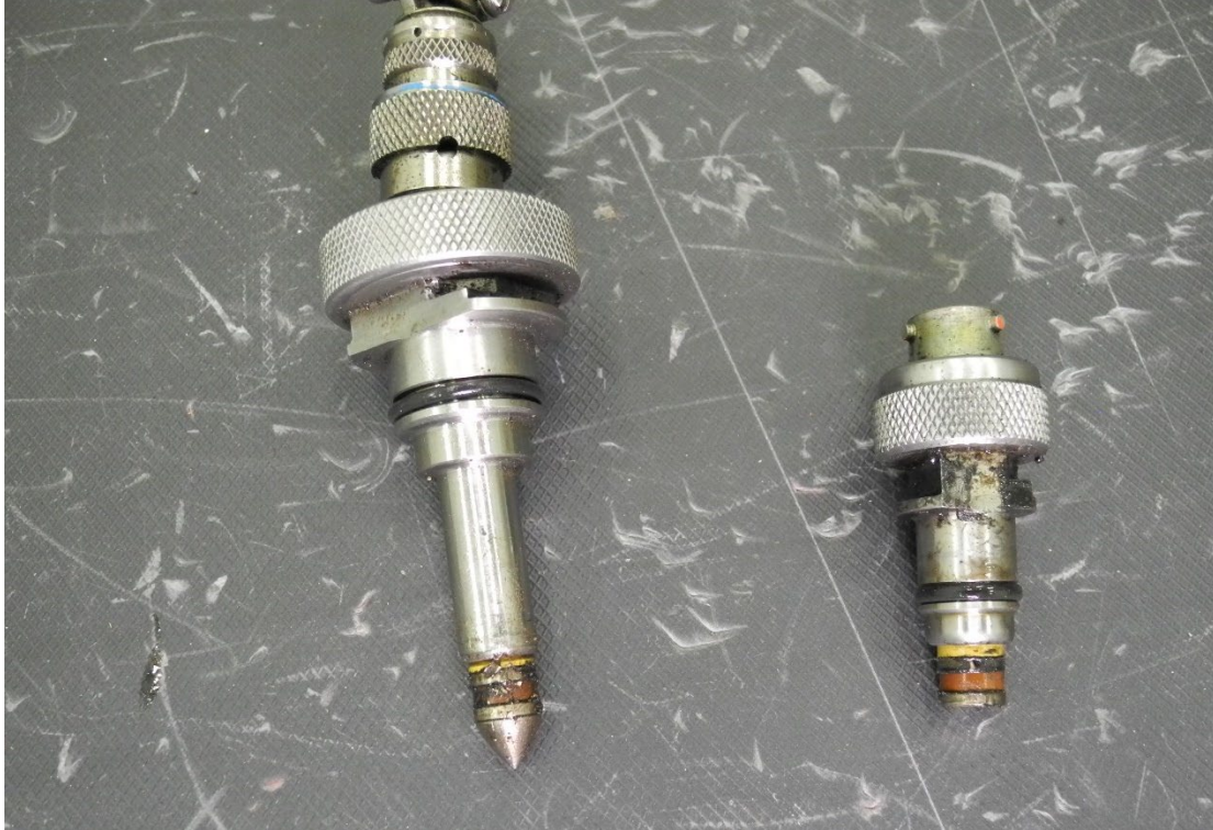
Photo 8 - Gearbox Oil Chip Detectors - Clean
