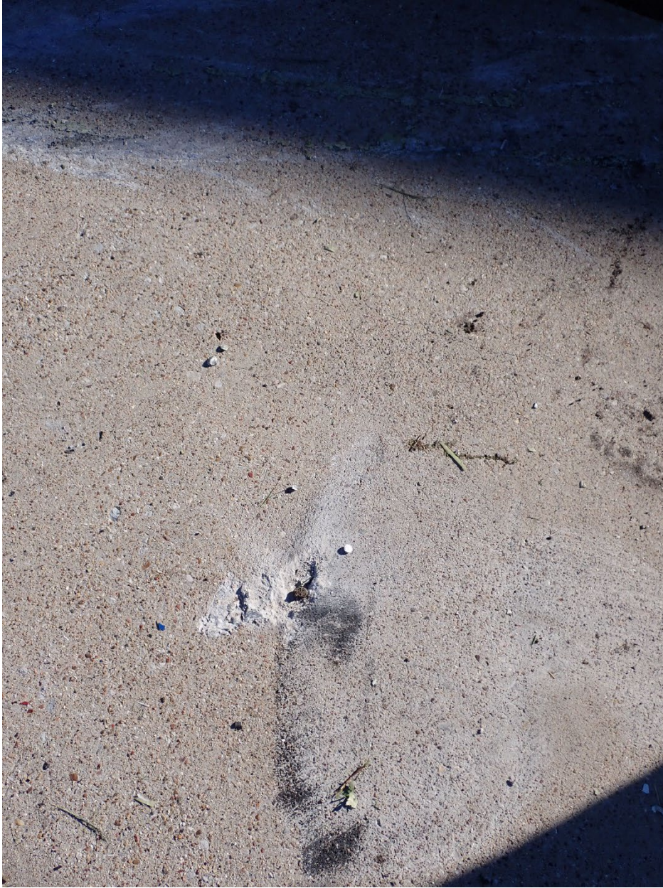
Figure 6: Right landing gear ground scar and witness mark
