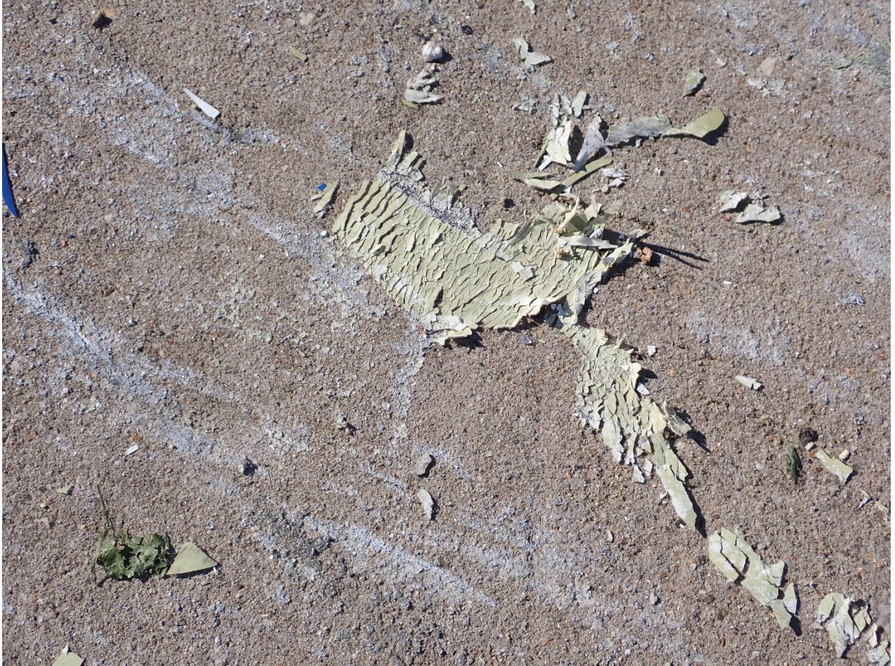
Figure 2: Leading edge paint transfer
