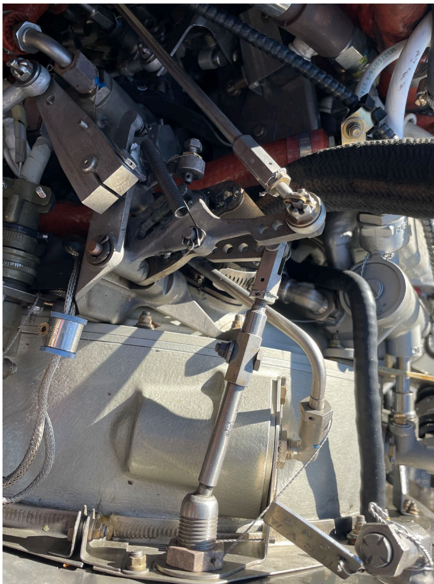
Photograph 4 - Engine Control Linkage
