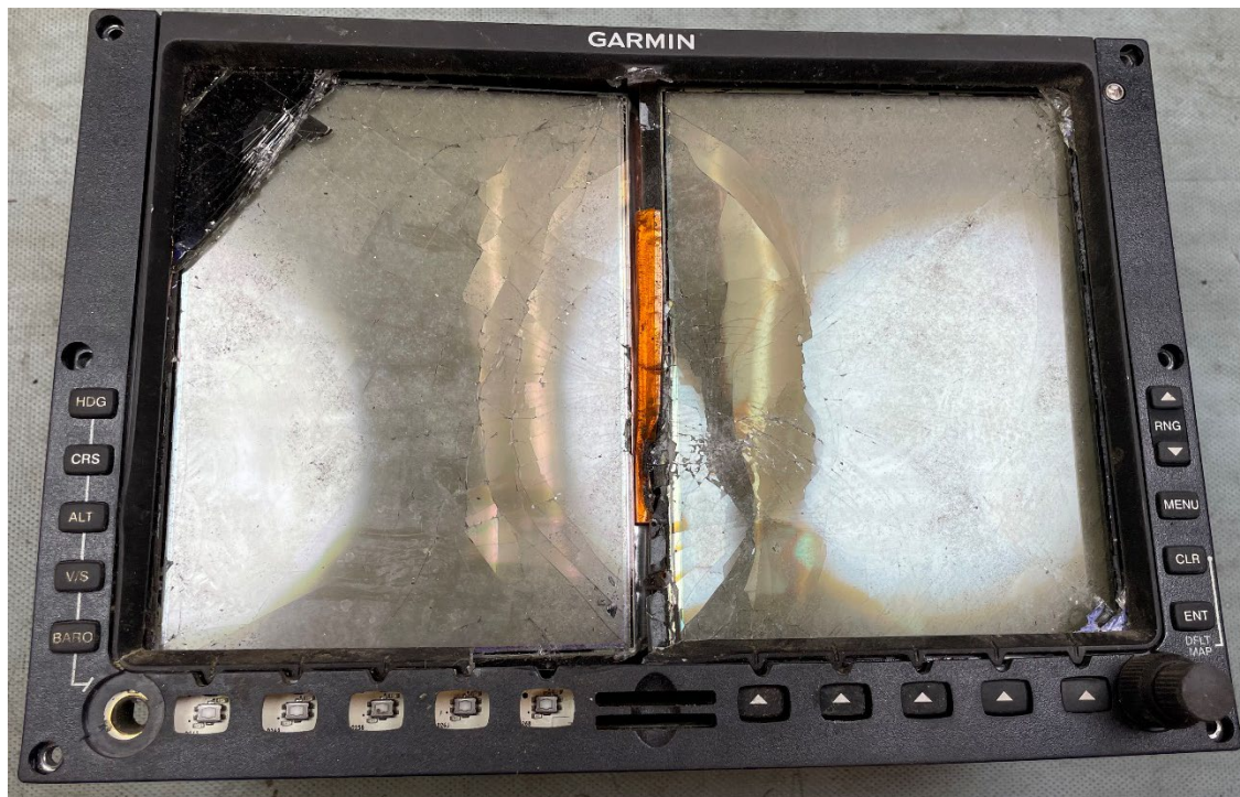
Figure 1. Garmin GDU 620 as received by the NTSB Vehicle Recorder Laboratory.
