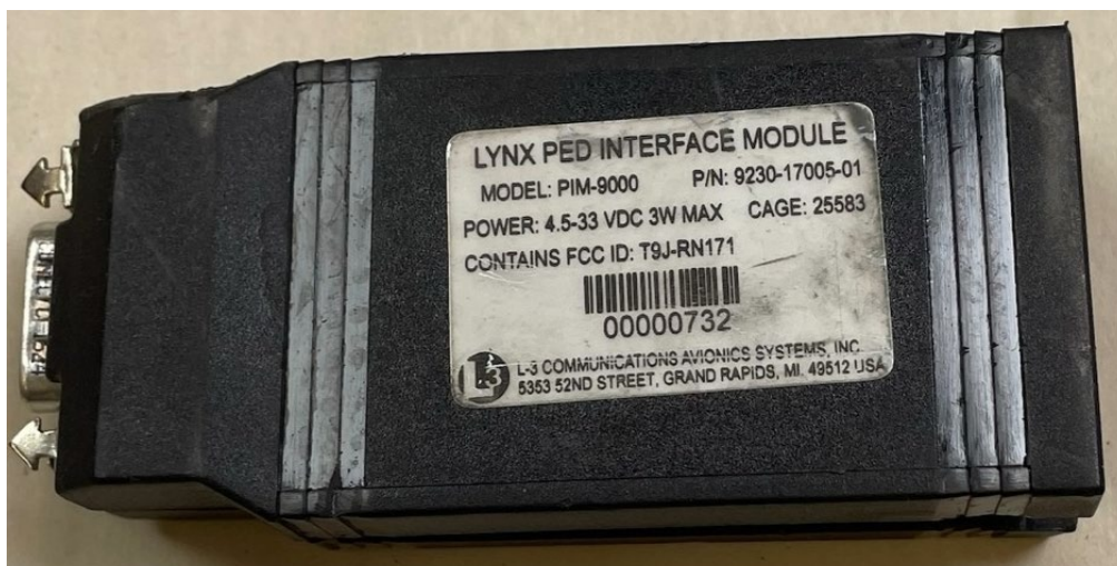
Figure 5. L-3 Lynx PED Interface Module PIM-9000 as received by the NTSB Vehicle Recorder Laboratory.
