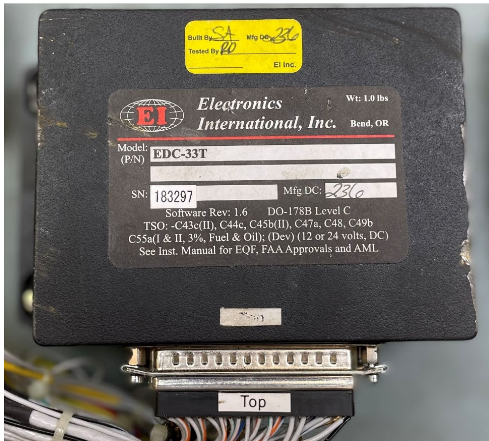
Figure 3. EI EDC-33T as received by the NTSB Vehicle Recorder Laboratory.
