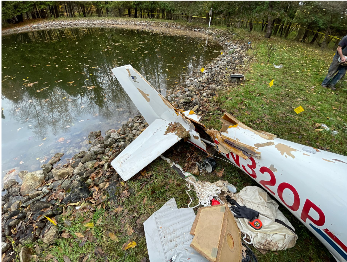
Photograph 3 - Aft fuselage during examination (NTSB Photo)
