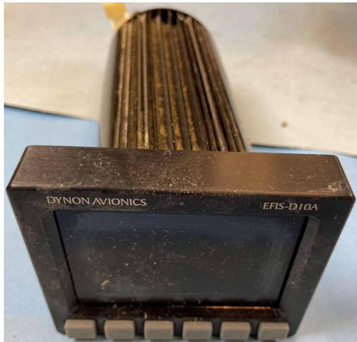
Figure 3. Dynon EFIS-D10A as received by the NTSB Vehicle Recorder Laboratory.
