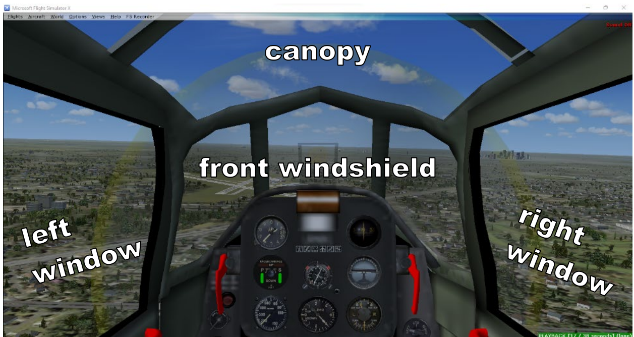
Figure 23. Exemplar P-63 cockpit interior in Microsoft Flight Simulator. Window terminology for this report is shown.
