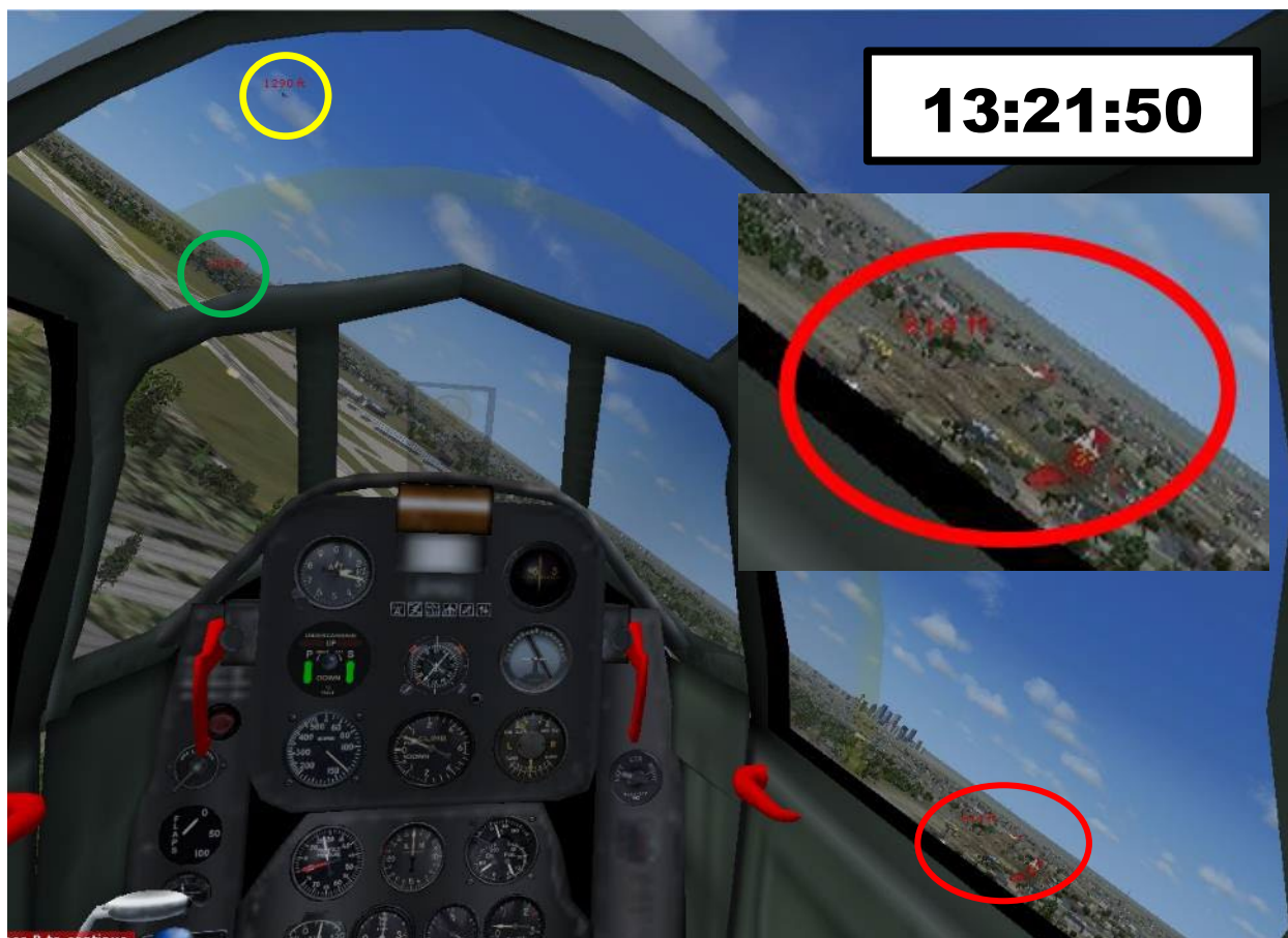
Figure 28. View of the lead P-51 (circled in yellow), the second P-51 (circled in green) and B-17 (circled in red) from exemplar P-63 cockpit interior in Microsoft Flight Simulator at 13:21:50. This is the final view of the B-17 from the P-63.
