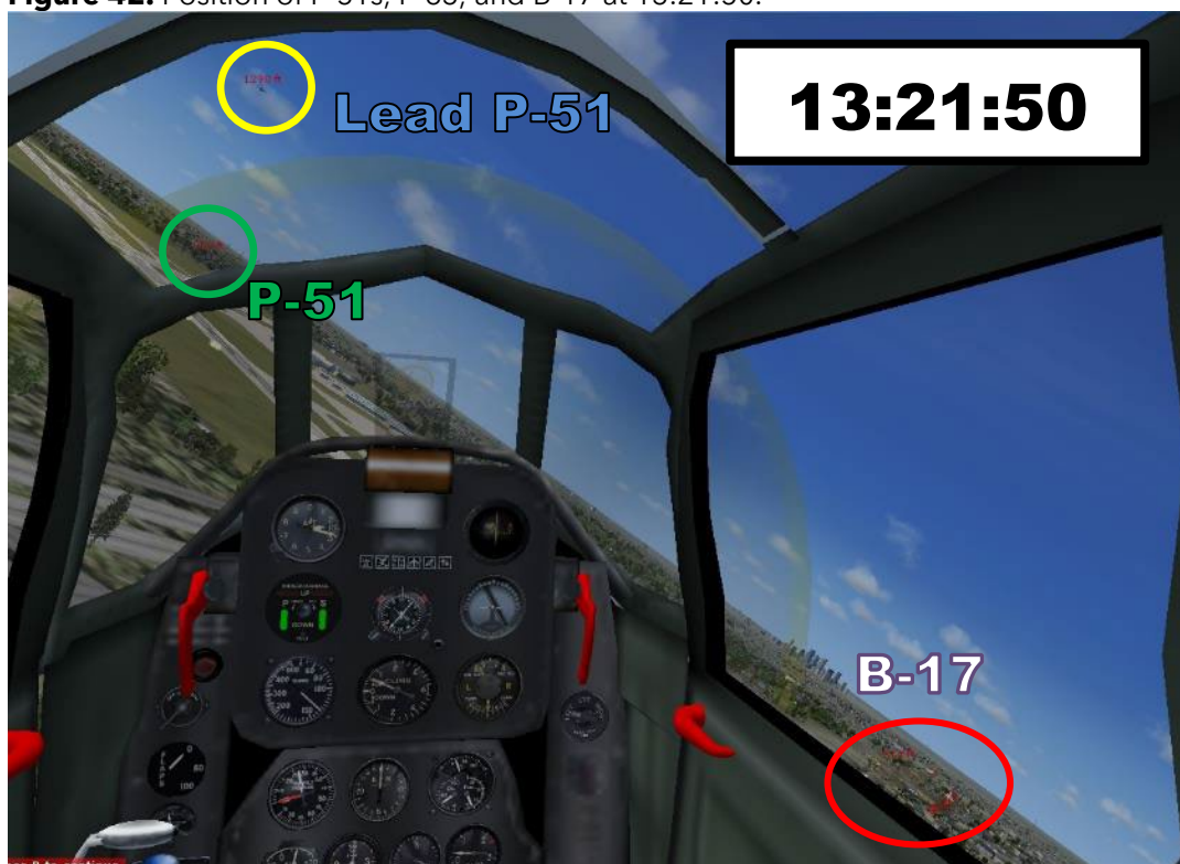
Figure 43. View of the lead P-51 (circled in yellow), the second P-51 (circled in green) and B-17 (circled in red) from exemplar P-63 cockpit interior in Microsoft Flight Simulator at 13:21:50. This is the final view of the B-17 from the P-63.
