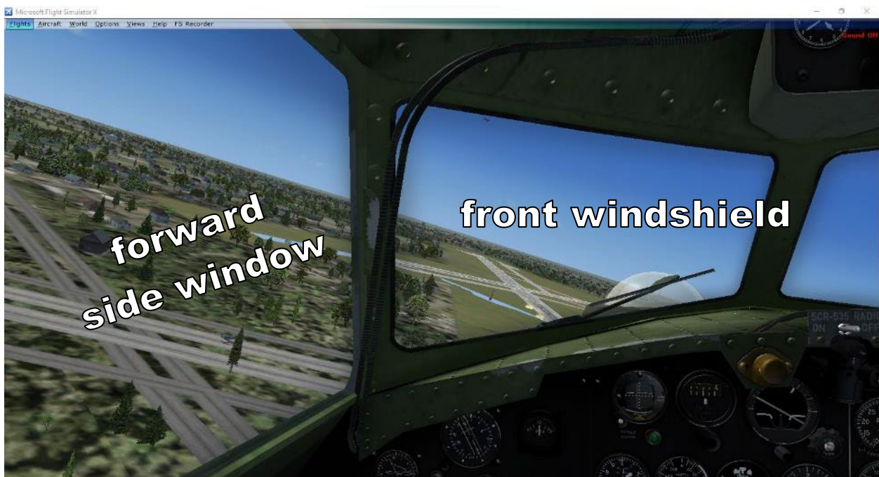
Figure 31. Forward view from the pilot's seat of exemplar B-17 cockpit interior in Microsoft Flight Simulator. The view must be turned to the left to see out the aft side window.
