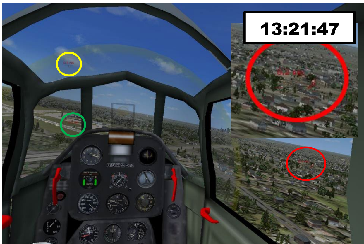
Figure 27. View of the lead P-51 (circled in yellow), the second P-51 (circled in green) and B-17 (circled in red) from exemplar P-63 cockpit interior in Microsoft Flight Simulator at 13:21:47.
