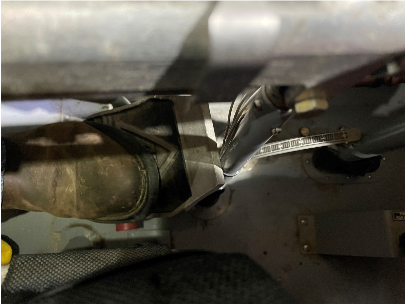
Photograph 8 - Spray valve pushrod and rudder pedal (Courtesy of NTSB)
