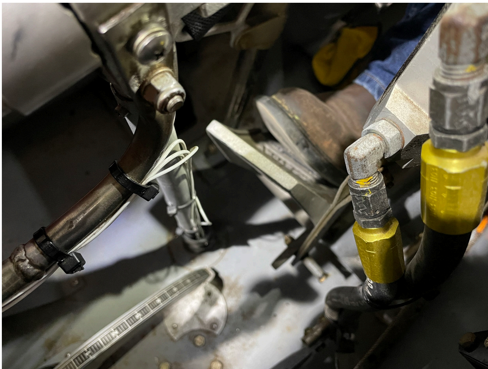
Photograph 6 - Spray valve lever and rudder pedal (Courtesy of NTSB)
