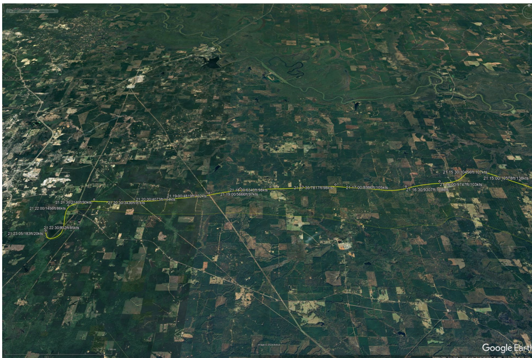
Figure 5. Google Earth overlay of approximately the final 10 minutes of the accident flight recorded on the Garmin GDU 1060. MSL Altitude and Groundspeed are depicted.
