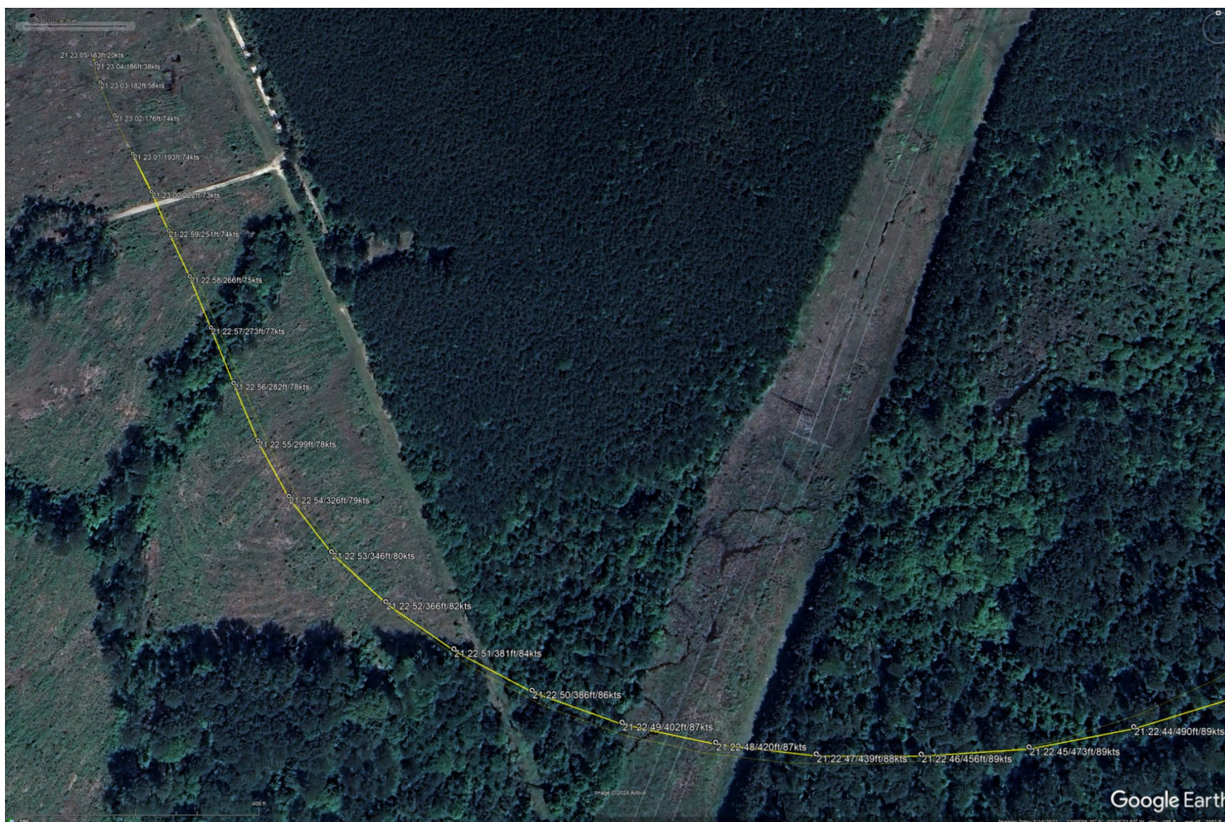
Figure 6. Google Earth overlay of approximately the final 20 seconds of the accident flight recorded on the Garmin GDU 1060. MSL Altitude and Groundspeed are depicted.
