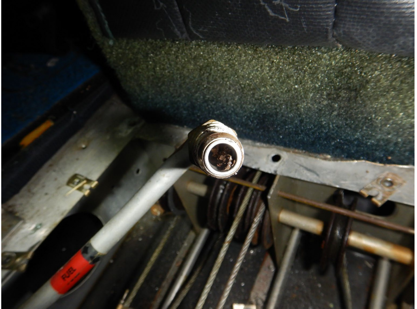
TAI Examination ASI-23-CU-050 (Left Fuel Line Debris)
