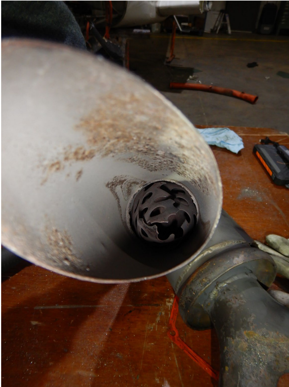
TAI Examination ASI-23-CU-059 (Exhaust Baffle Obstructing Exhaust Exit)
