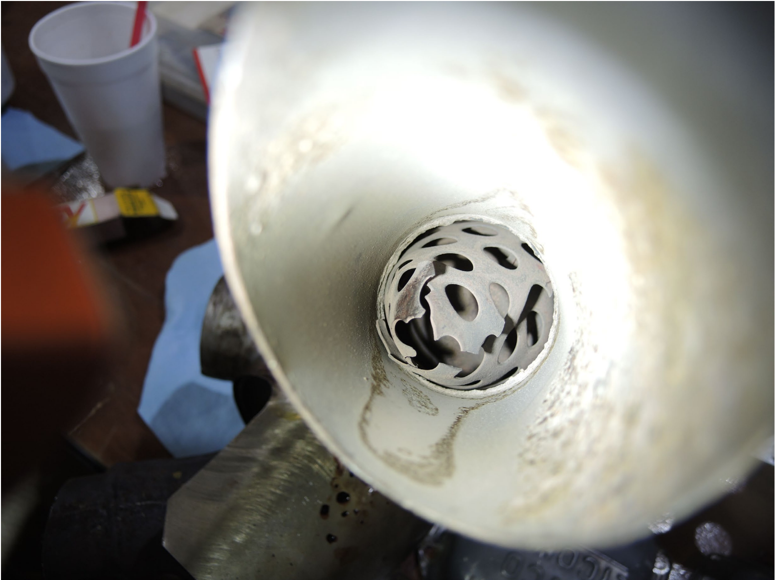
Photograph 9 - Tailpipe blockage (Courtesy of NTSB)
