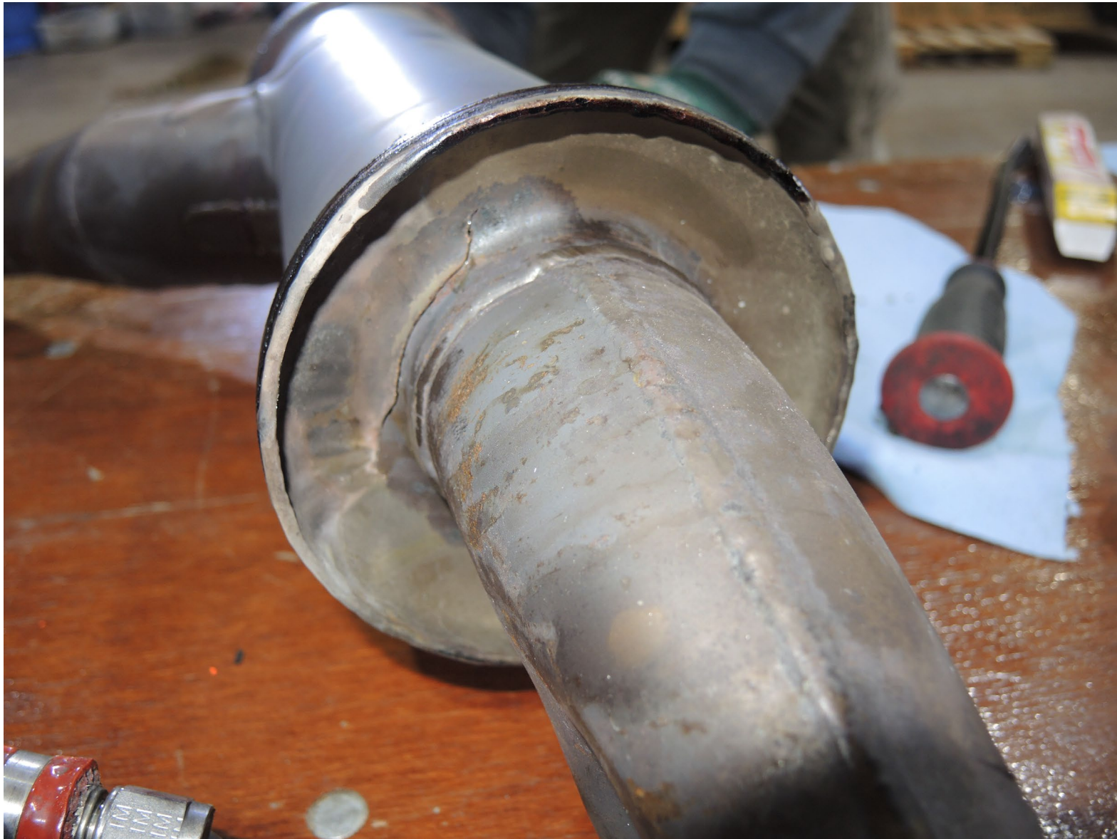
Photograph 7 - Muffler endcap crack (Courtesy of NTSB)
