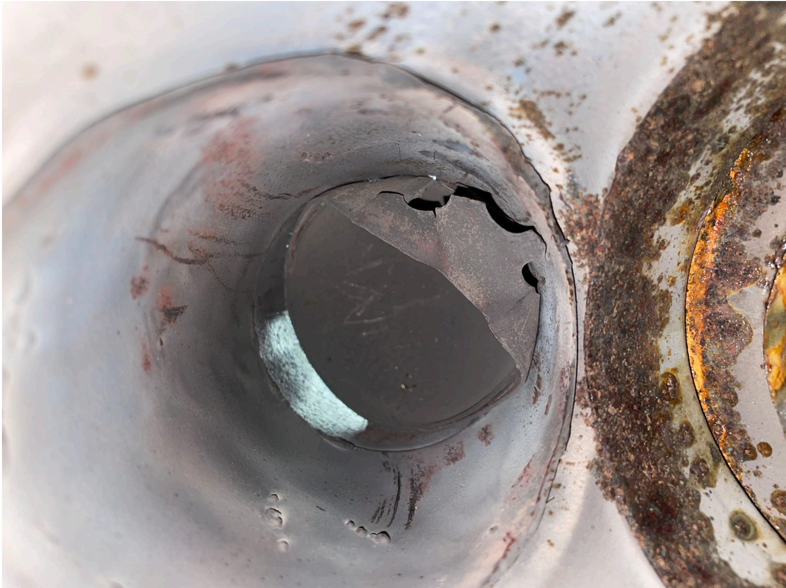
Photograph 12 - Flame tube lodged in tailpipe (Courtesy of NTSB)
