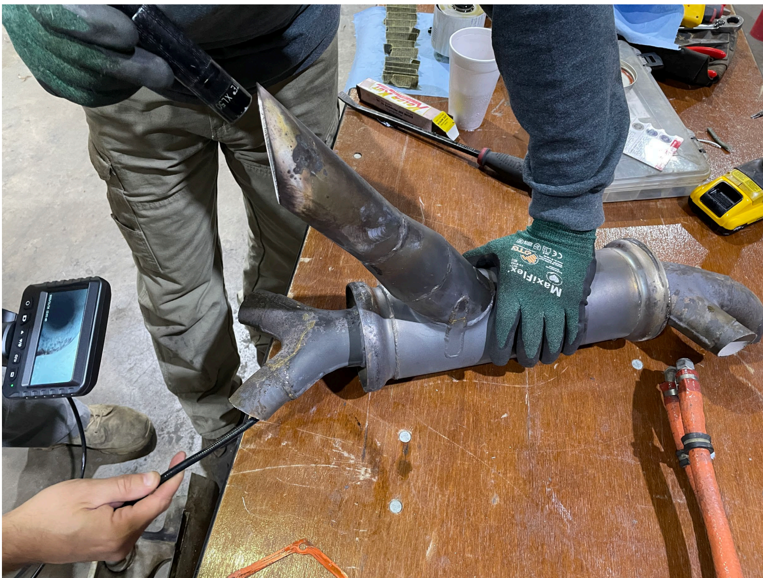
Photograph 8 - Muffler (Courtesy of NTSB)
