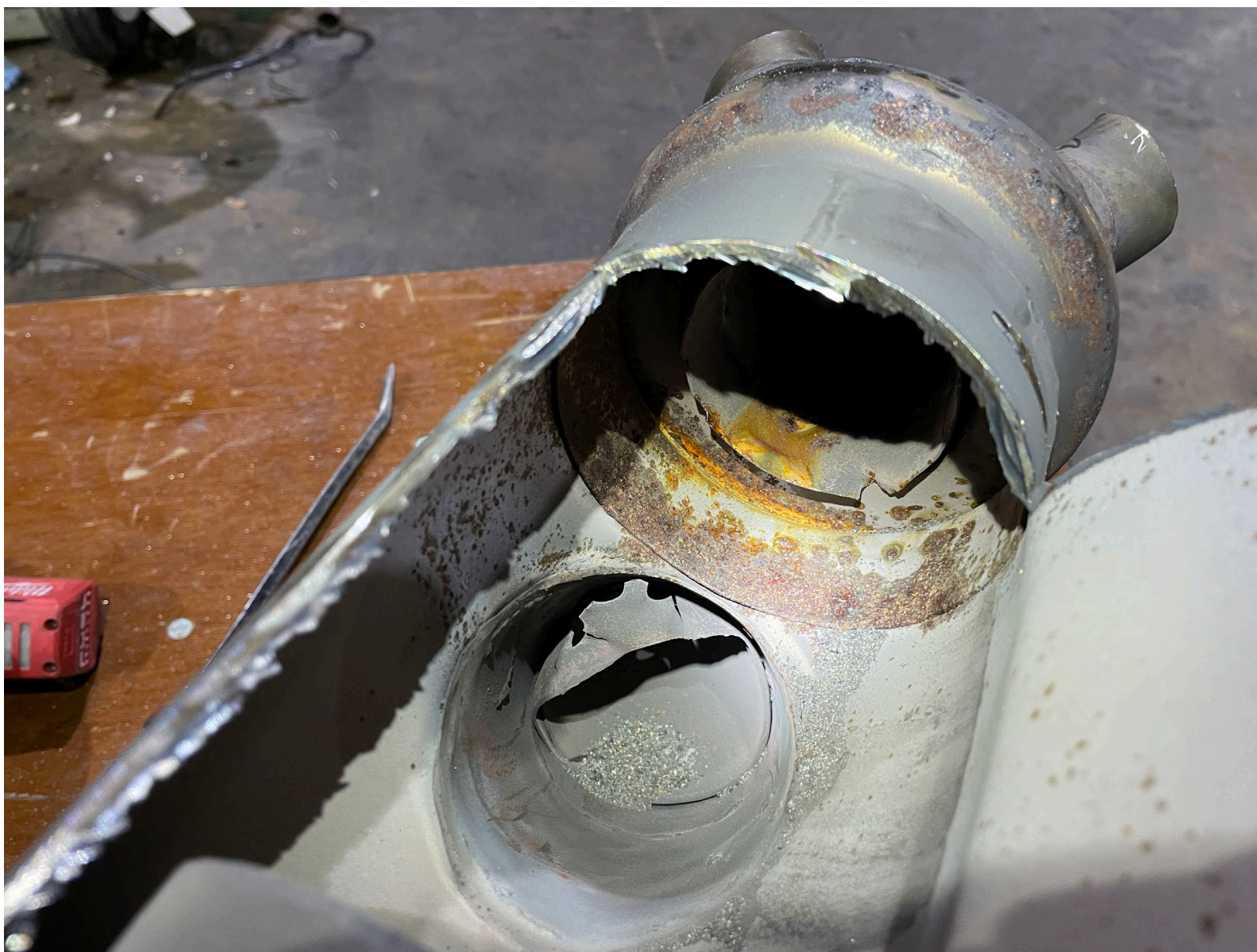
Photograph 10 - Inside muffler, flame tube lodged in tailpipe (Courtesy of NTSB)
