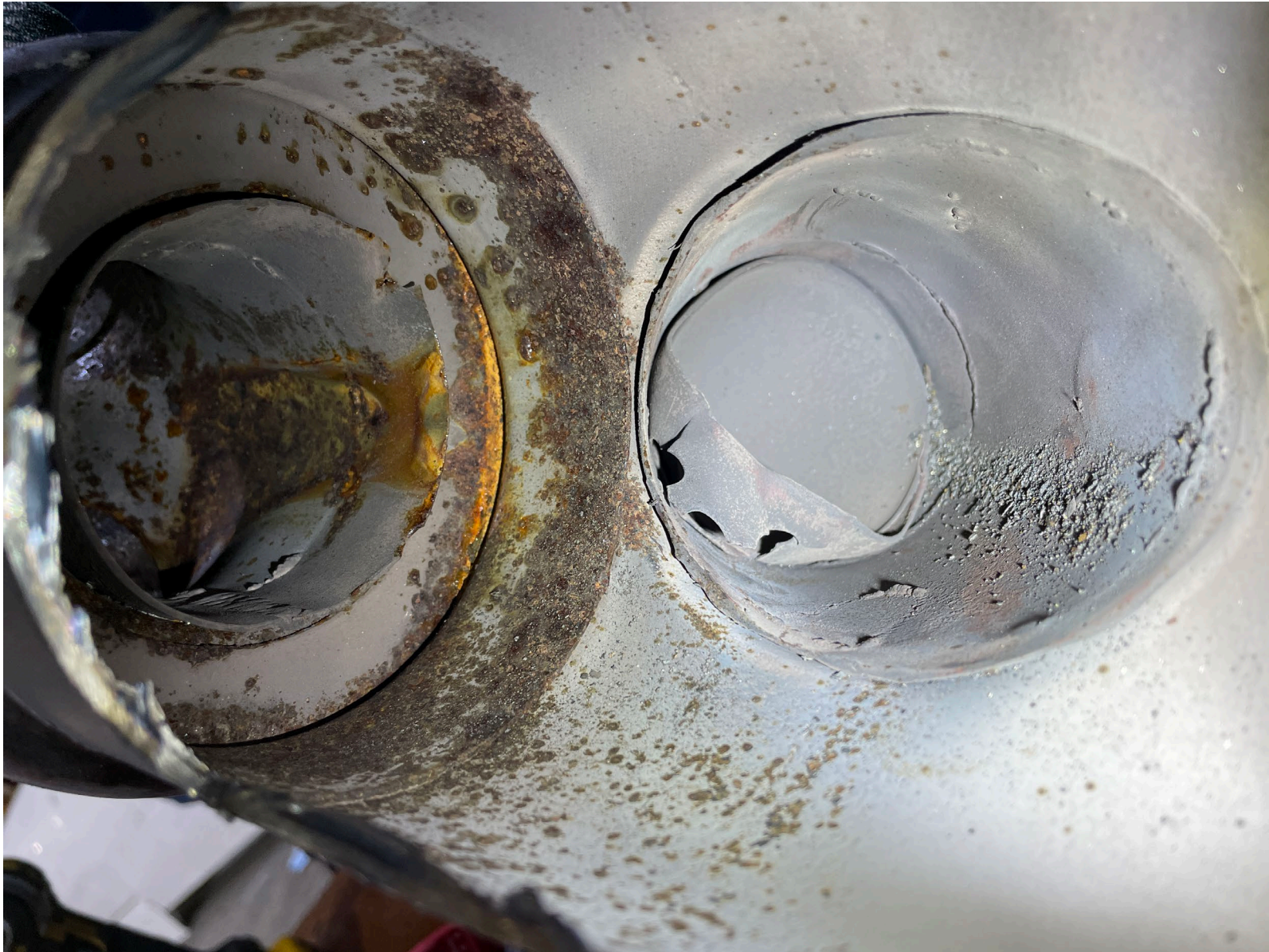
Photograph 11 - Inside muffler, flame tube lodged in tailpipe (Courtesy of NTSB)
