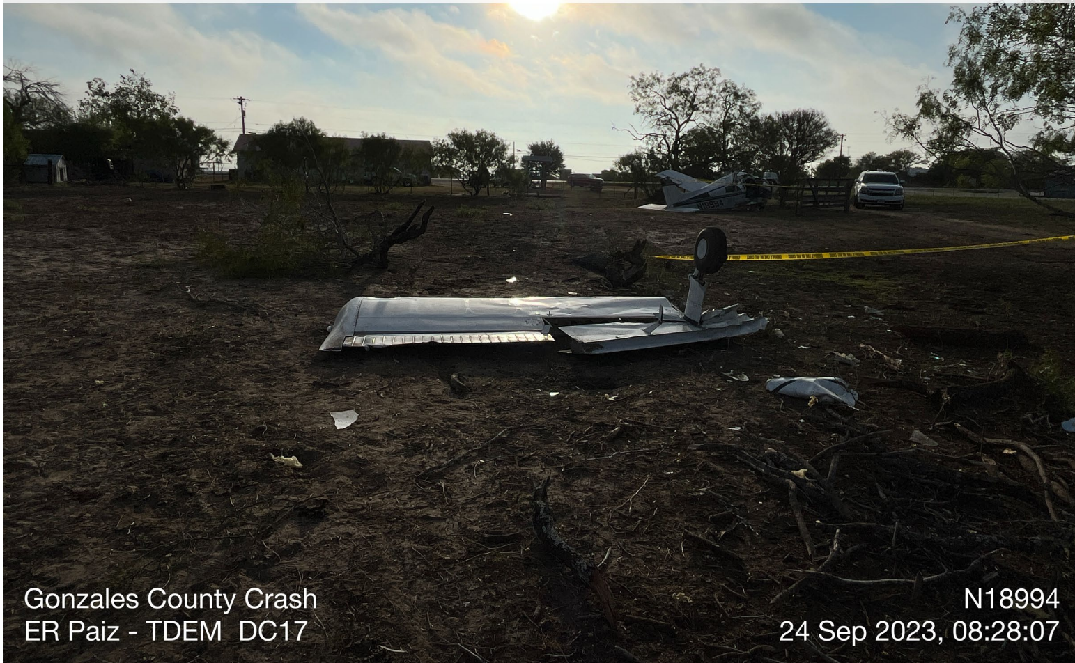
Photograph 2 - Separated right wing (Courtesy of Texas Emergency Management)
