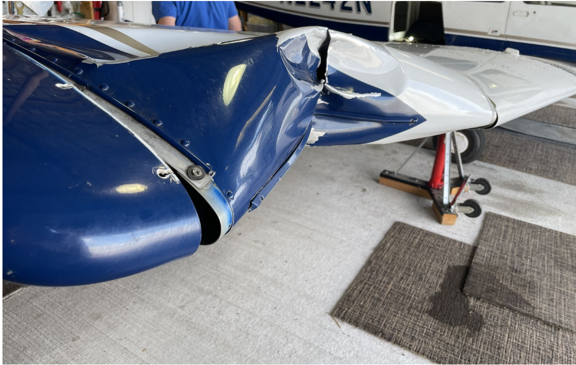
Photograph 2 - Outboard right wing damage (Courtesy of Federal Aviation Administration)
