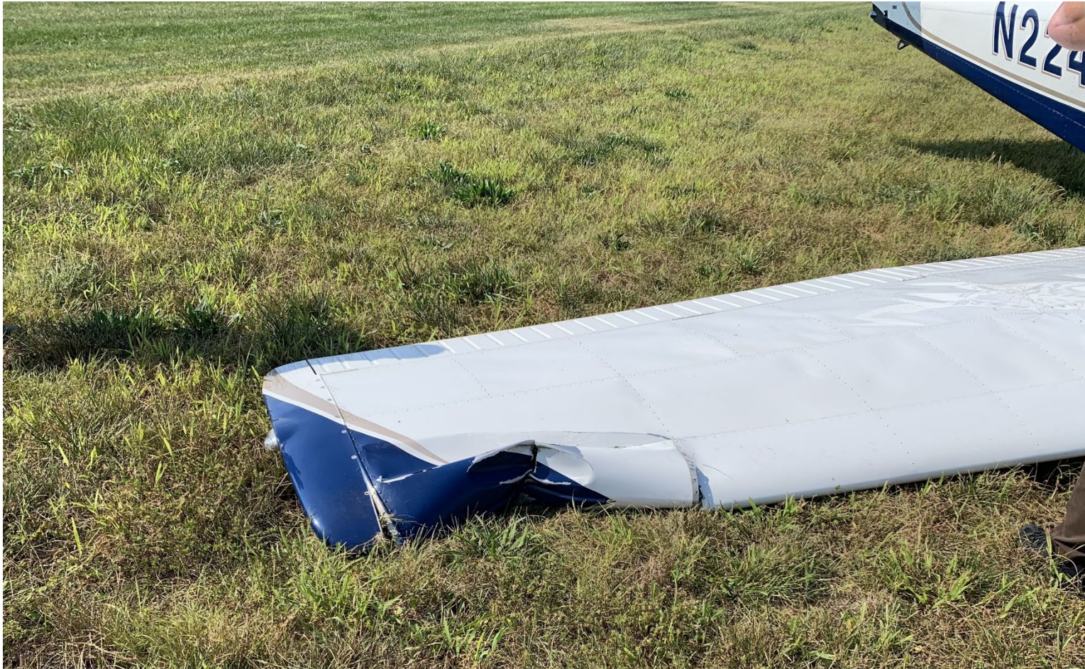
Photograph 1 - Outboard right wing damage (Courtesy of Federal Aviation Administration)
