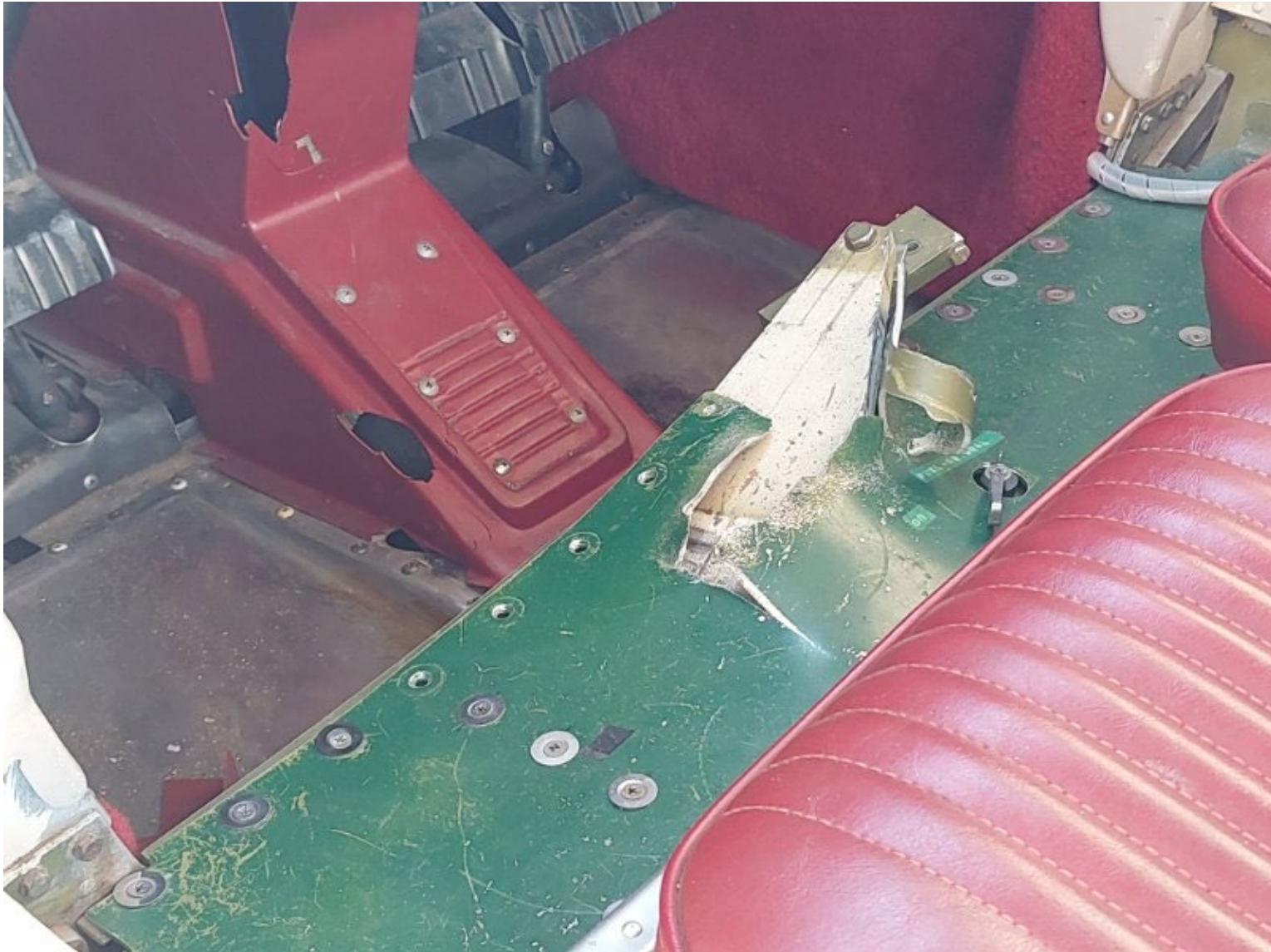
Photograph 1 - Left main landing gear strut punctured forward fuselage (Courtesy of Airport Operations)
